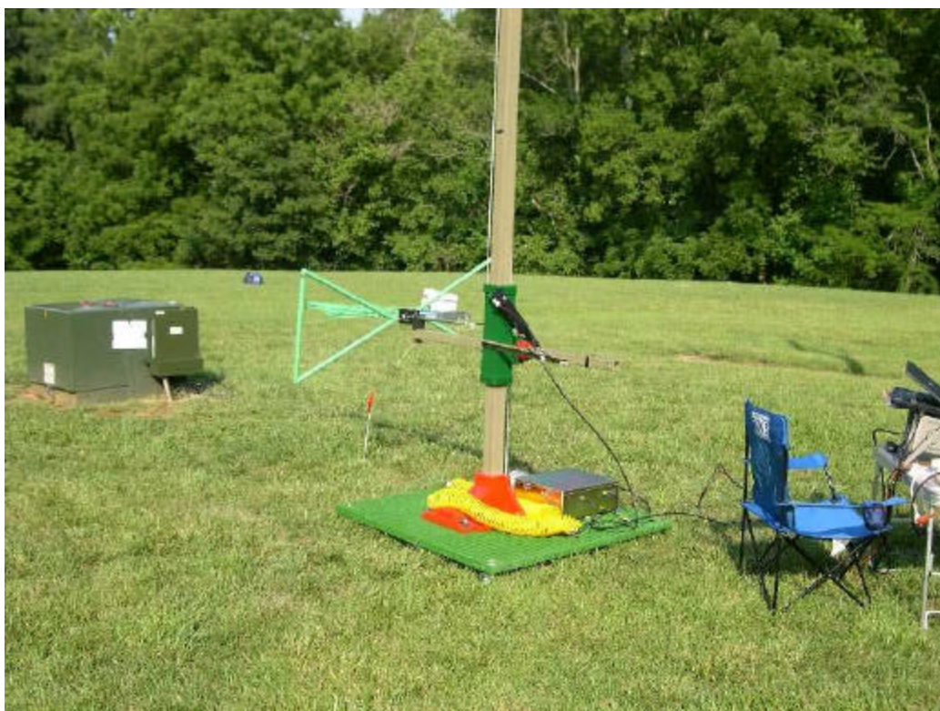
Radiated emissions measurement > 30 MHz and 3m
