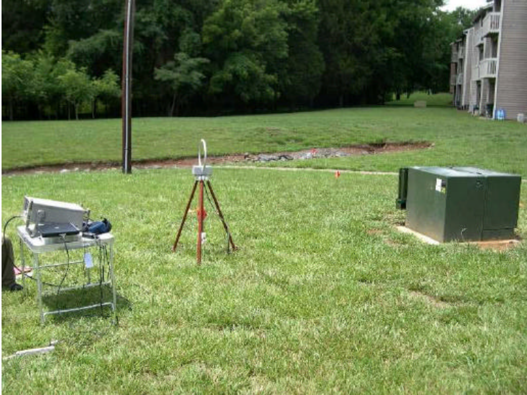
Radiated emissions measurement < 30 MHz and 3m
