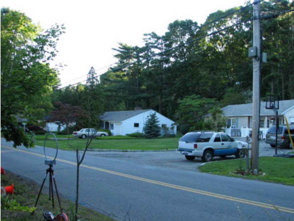
Radiated emission measurements < 30 MHz
