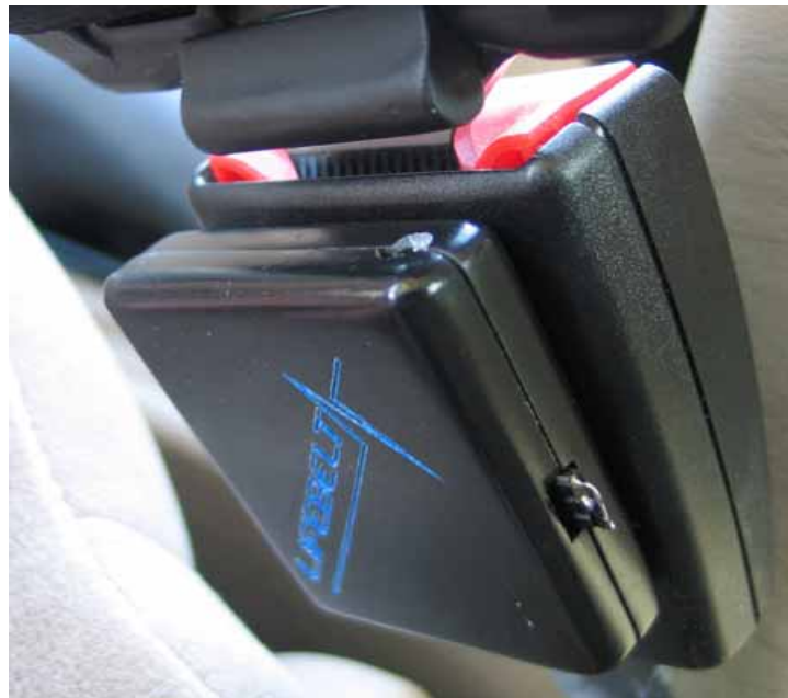
Figure 7. Typical Remote Switch Unit and Actuator mounting. *Repeat installation step for additional transmitters
