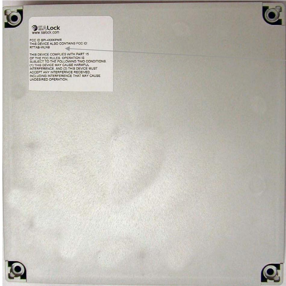
**Install the FCC label on the back of the plastic enclosure containing the PCB assembly in the upper left hand corner.**
