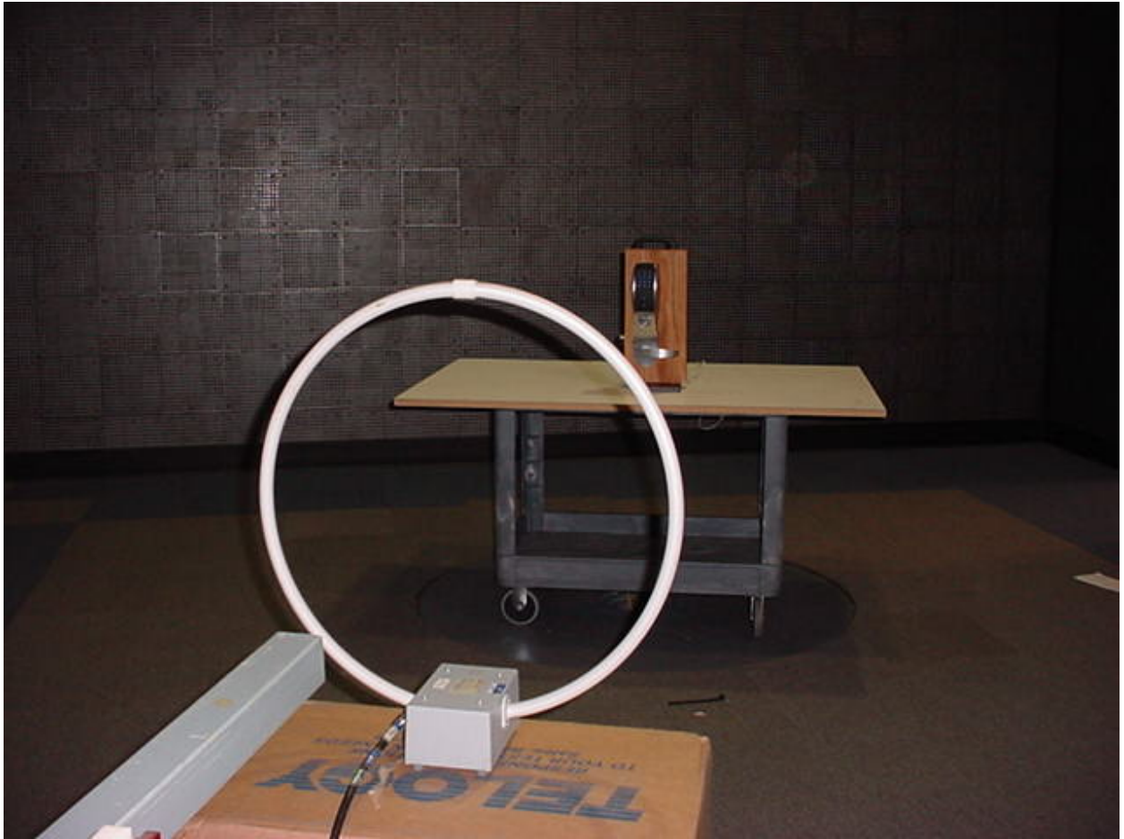
Figure 2: Radiated Emissions – Low Profile Enclosure (Front View)
