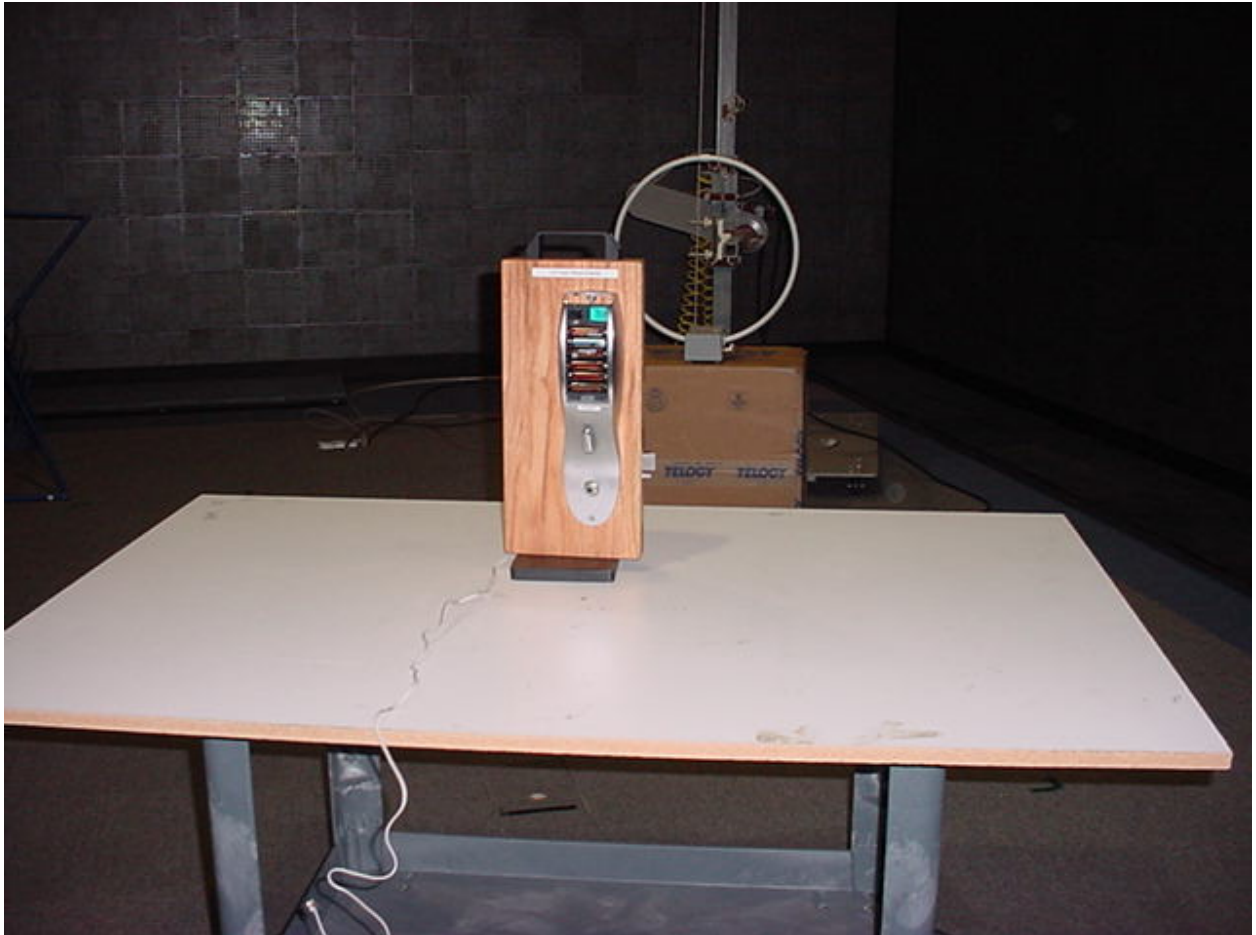
Figure 1: Radiated Emissions – Low Profile Enclosure (Rear View)
