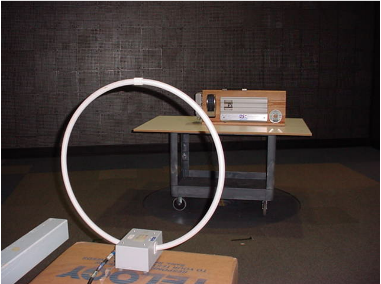
Figure 4: Radiated Emissions – Rollup Door Enclosure (Front View)
