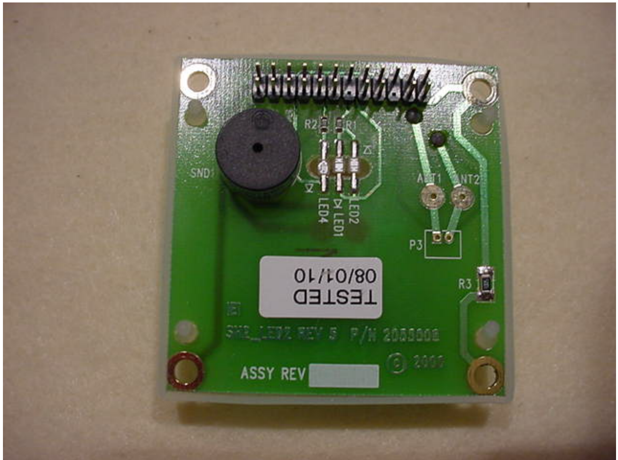
Figure 6: Transmitter Board (Rear View)
