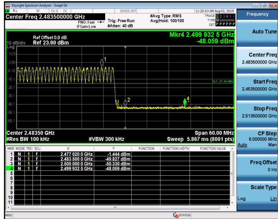
Band-edge for RF Conducted Emissions\_DH5\_2480\_Hopping Off
