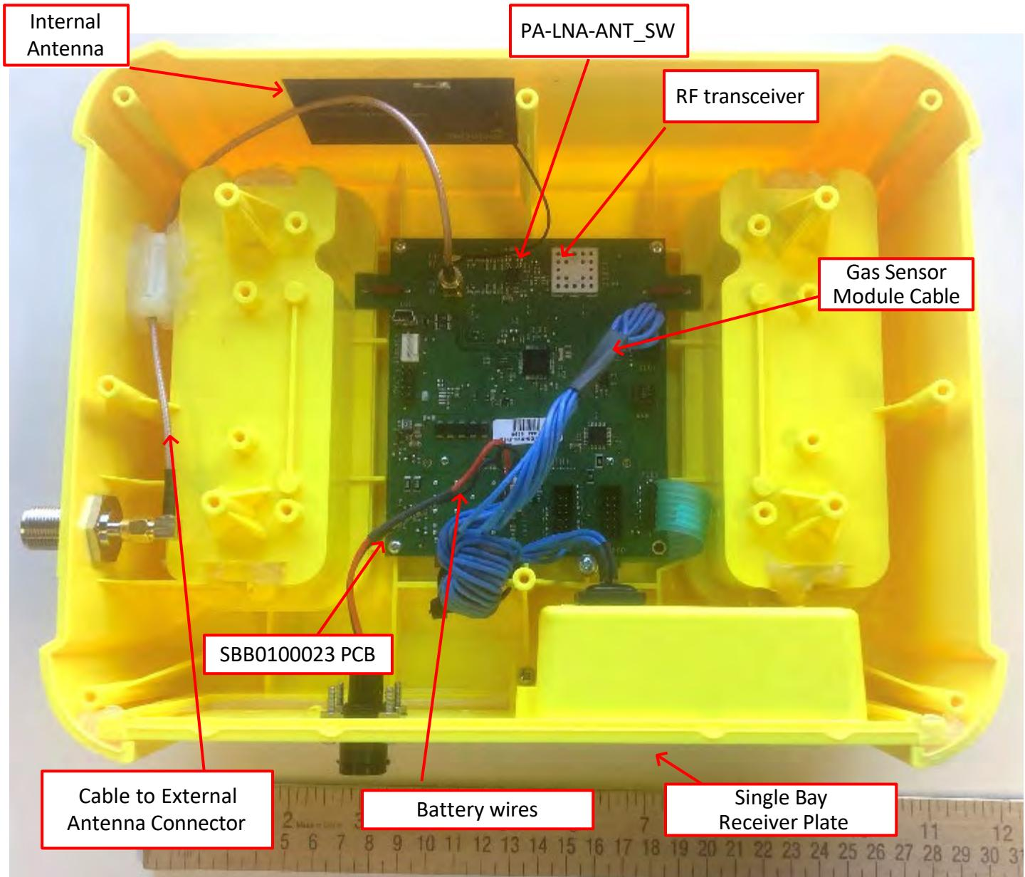
**FAP4913-090 WGM+ EXTERNAL BATTERY – BACK COVER REMOVED; RF SHIELD REMOVED**
