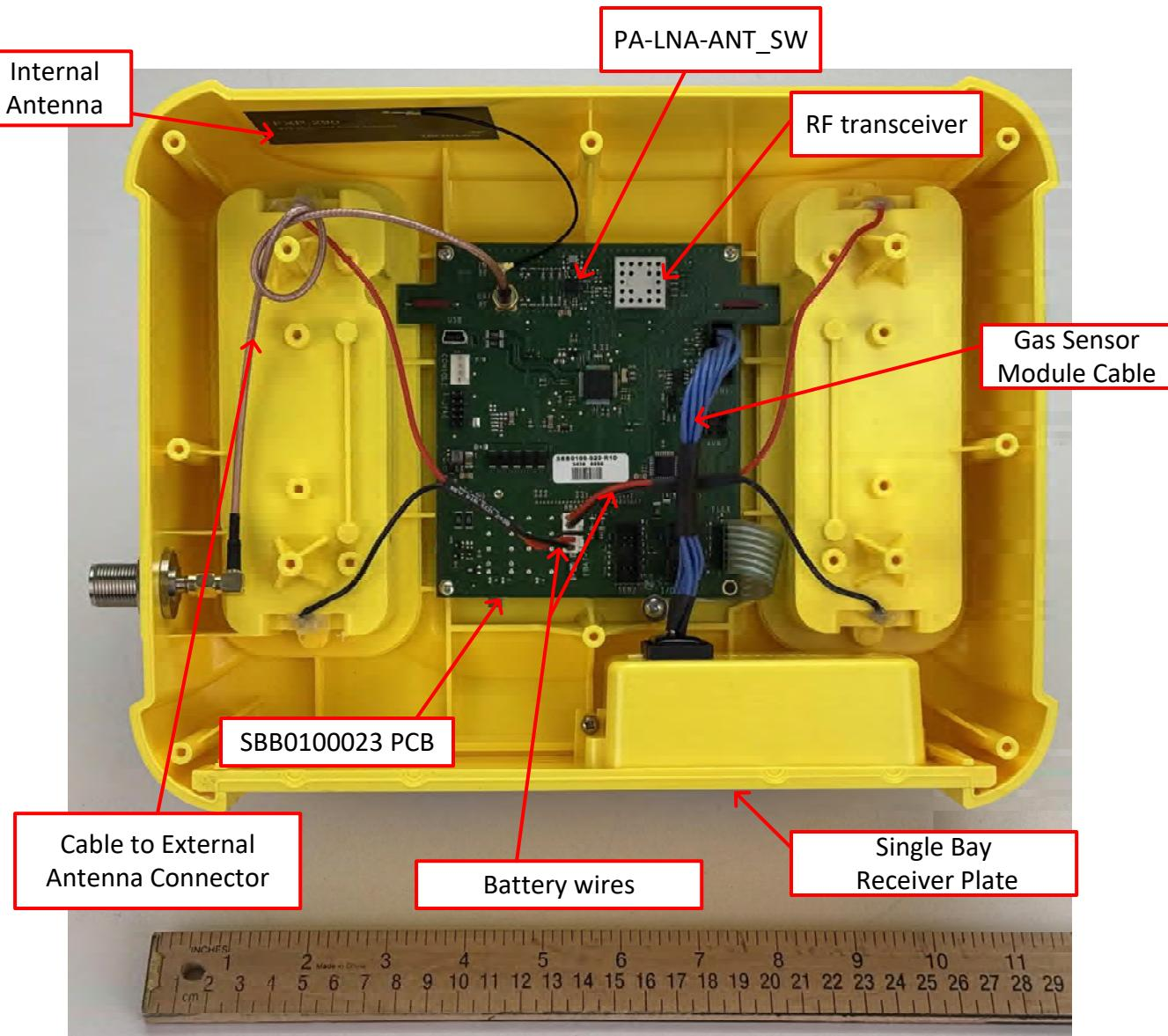
**FAP4913-030 WGM SINGLE BAY – BACK COVER REMOVED; RF SHIELD REMOVED**
