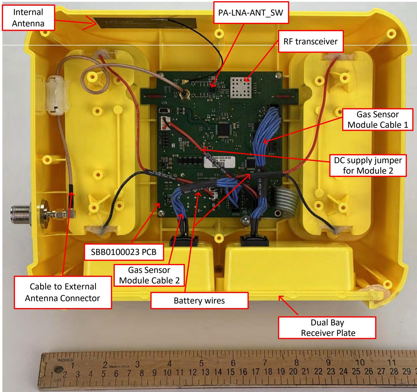
**FAP4913-032 WGM DUAL BAY – BACK COVER REMOVE; RF SHIELD REMOVED**
