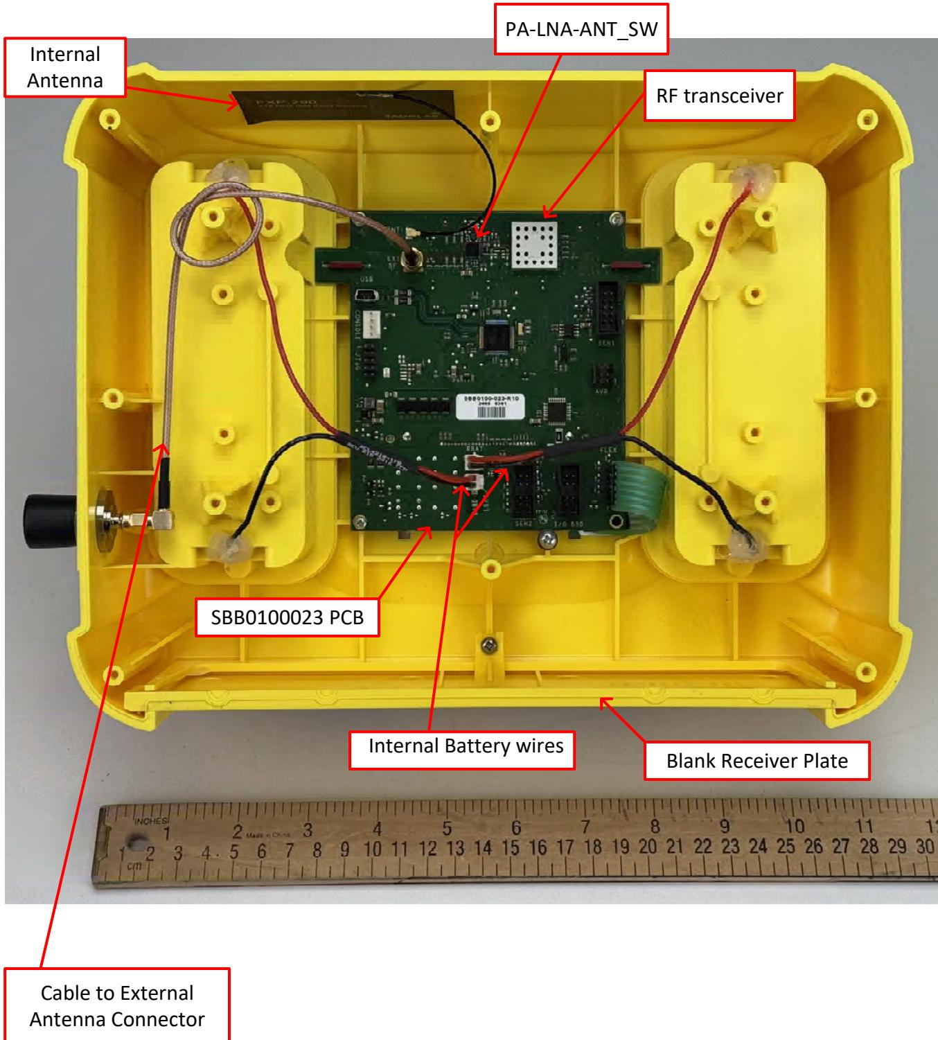
**FAP4213-093 BMN with INTERNAL BATTERIES – BACK COVER REMOVED; RF SHIELD REMOVED**
