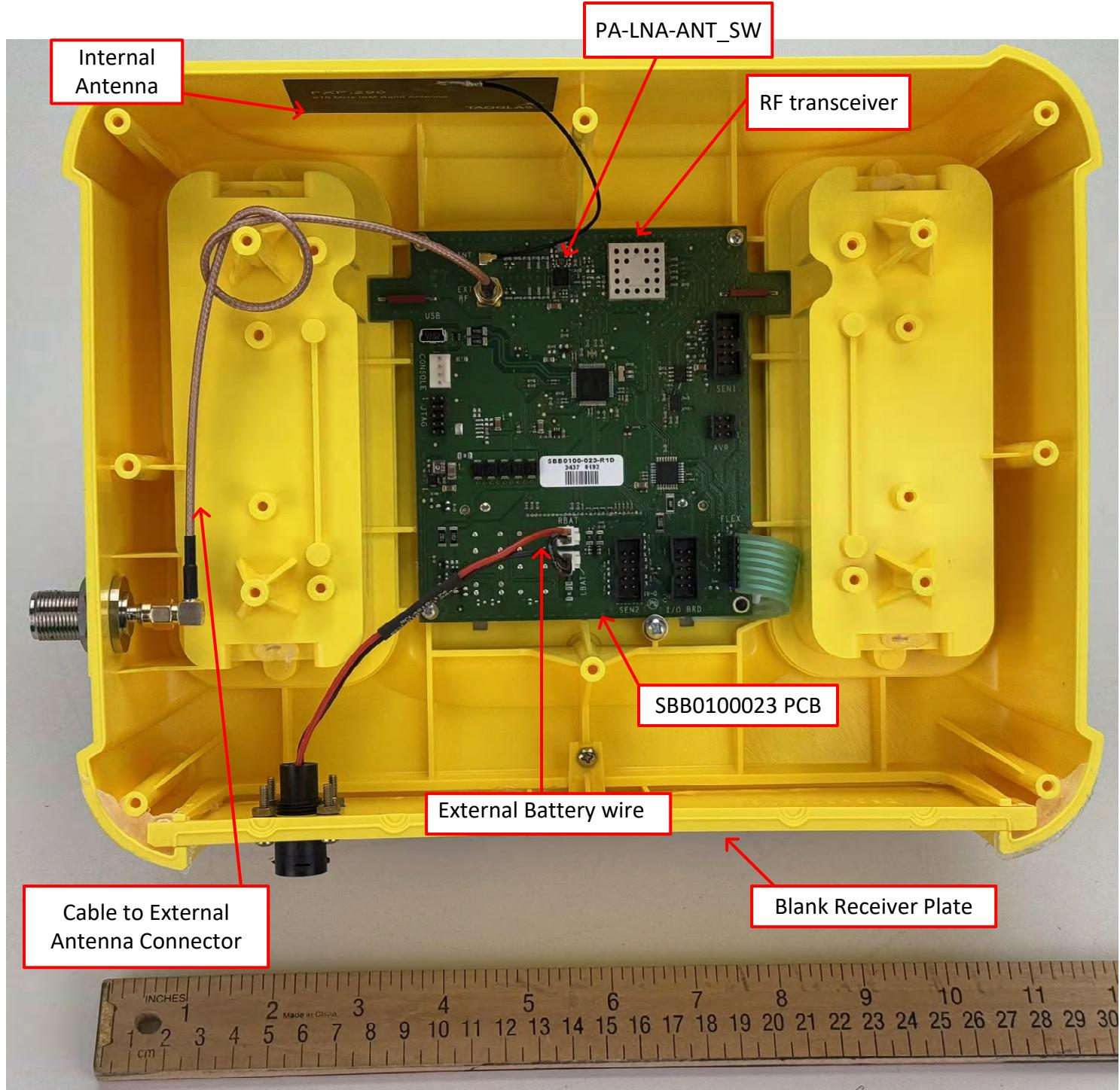
**FAP4213-090 BMN with EXTERNAL BATTERY – BACK COVER REMOVED; RF SHIELD REMOVED**
