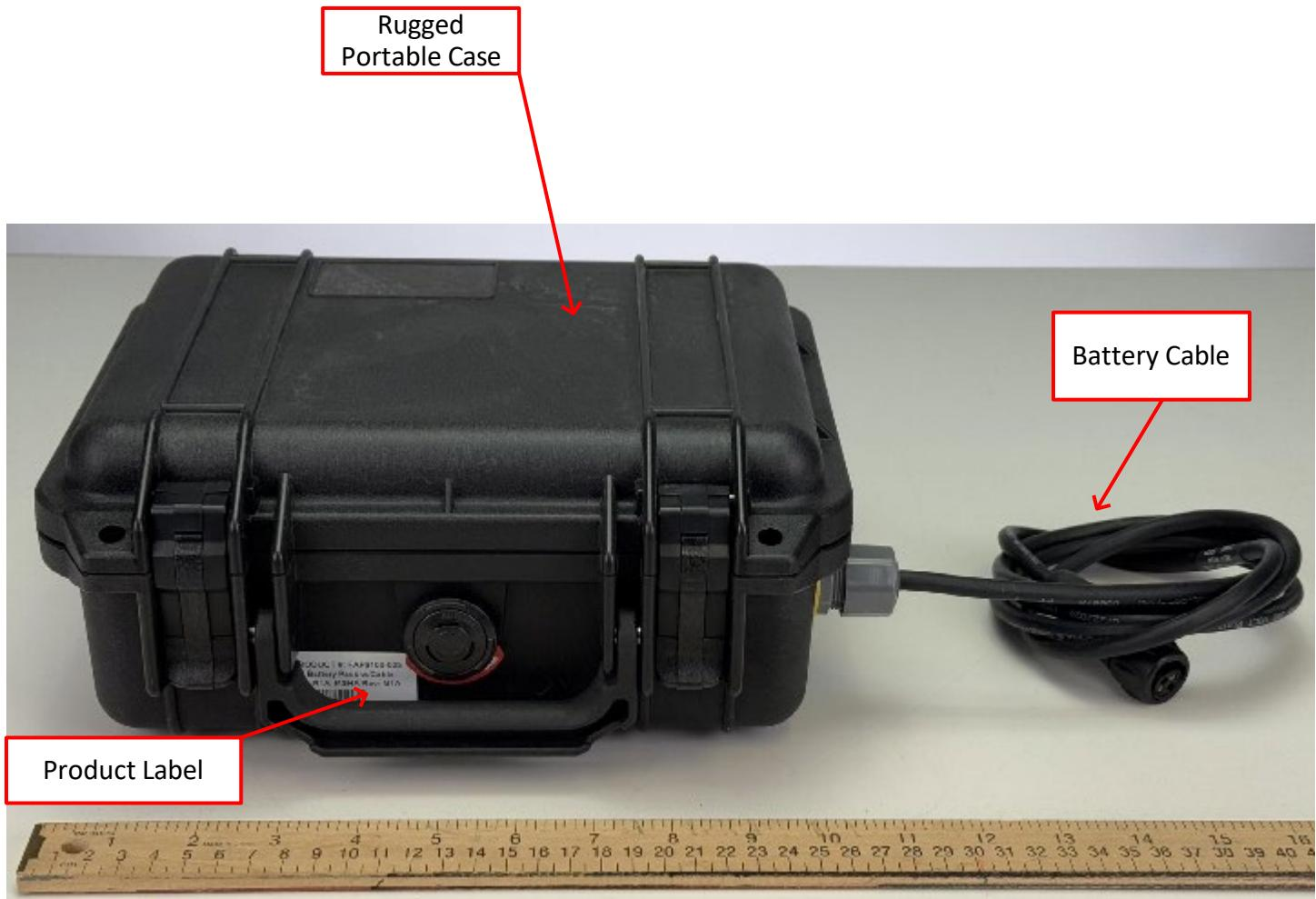
FAP9100-035 External battery can be used with the products tabulated below.
