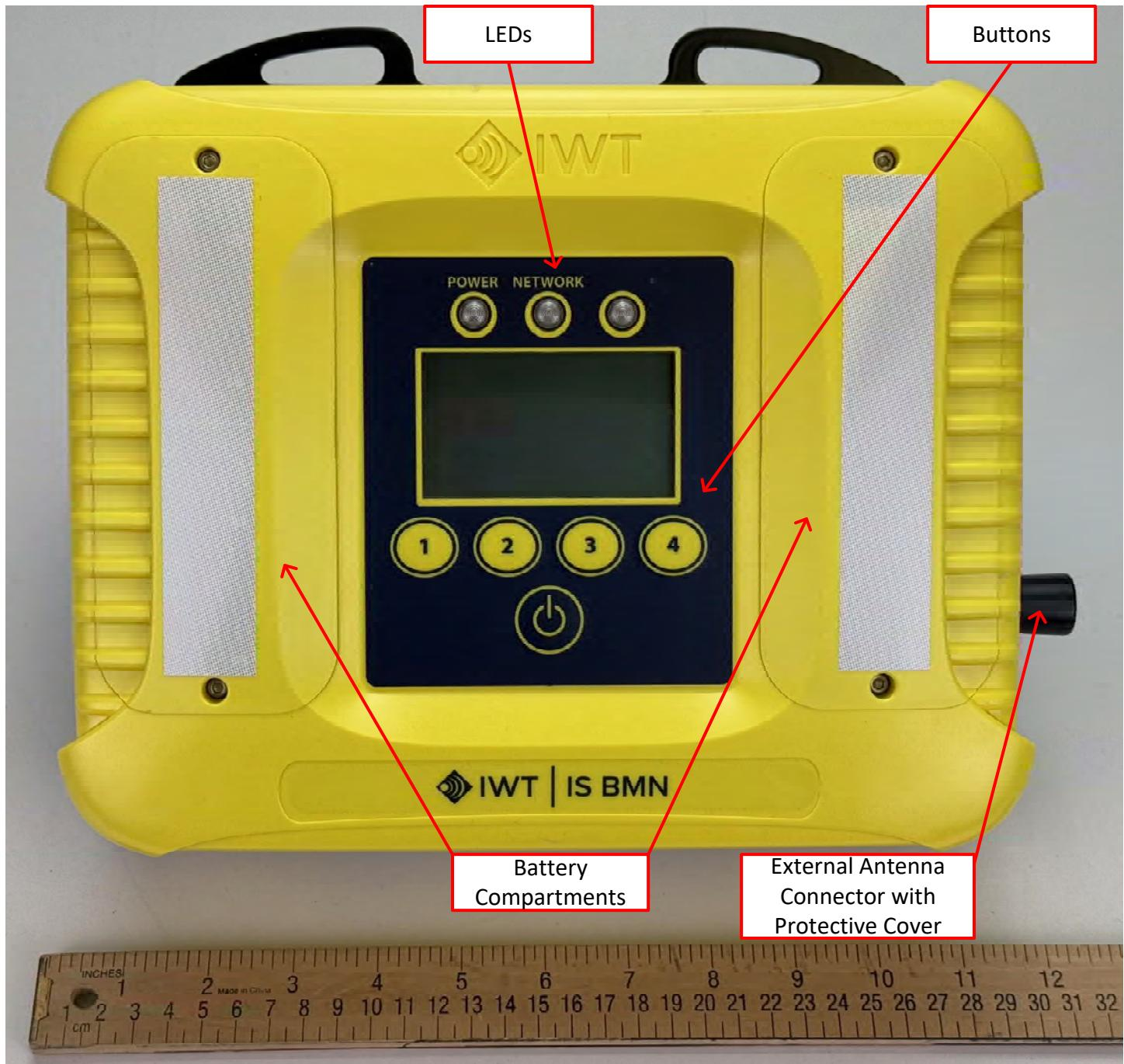
**FAP4213-093 BMN with INTERNAL BATTERIES – FRONT VIEW – BATTERY COOMPARTMENTS OPEN**
