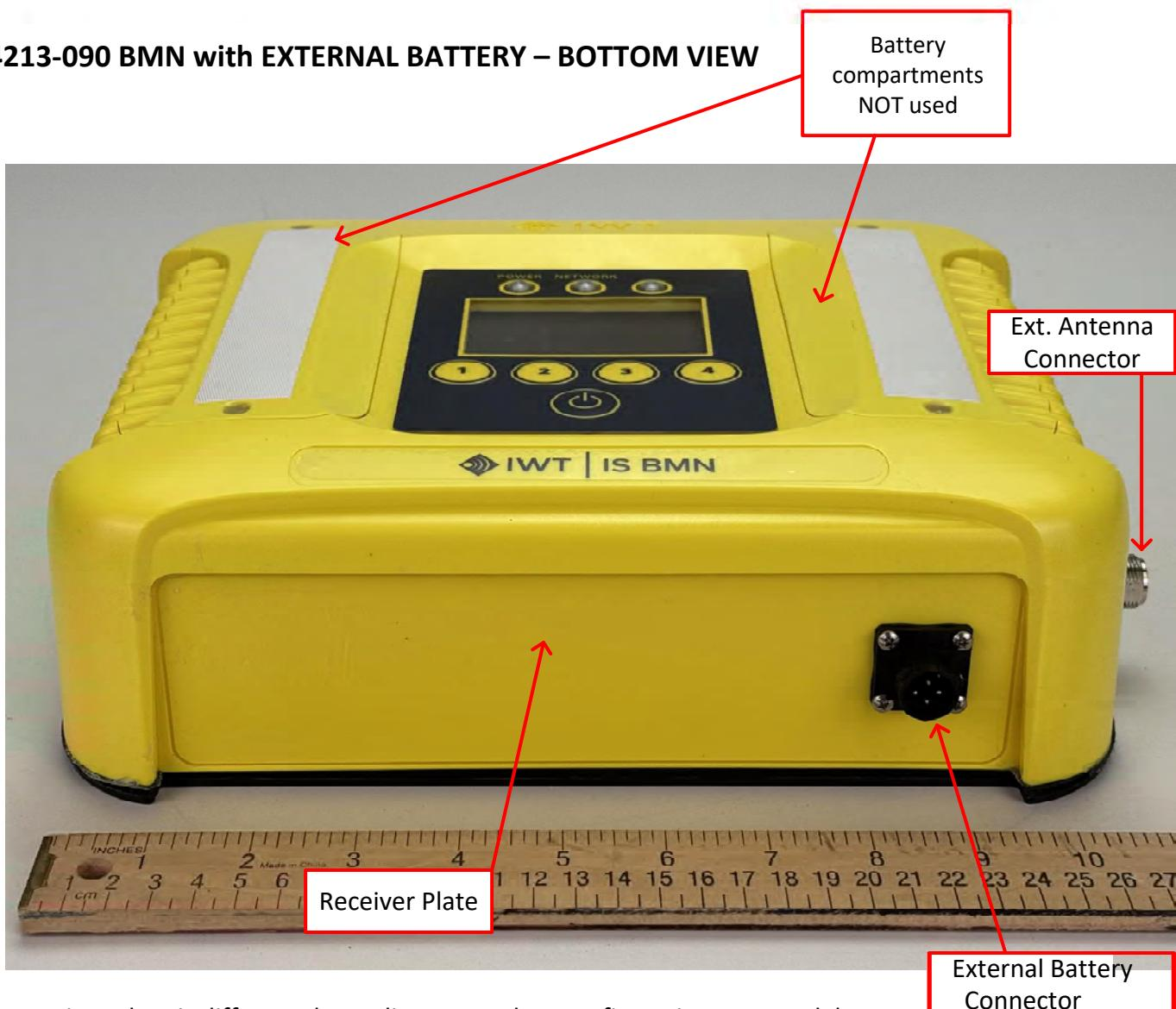
Receiver Plate is different depending on product configuration. For Model FAP4213-090 it is blank (solid) with an external battery connector.
