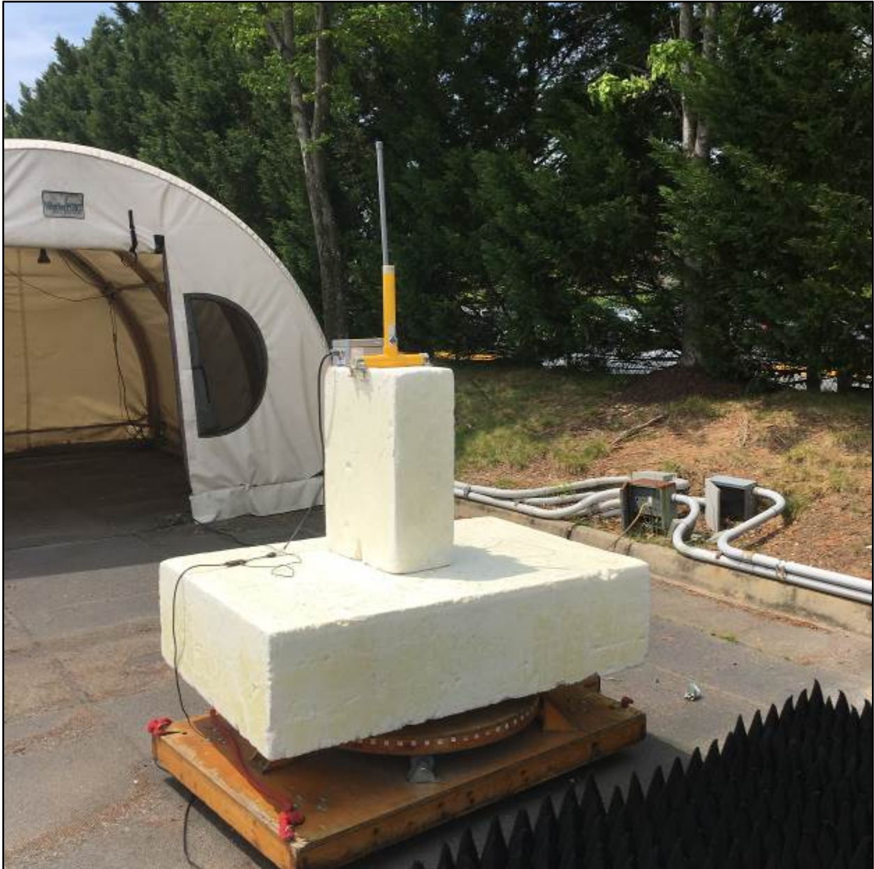
Photograph 5: Omni Antenna - Front View (Above 1 GHz)
