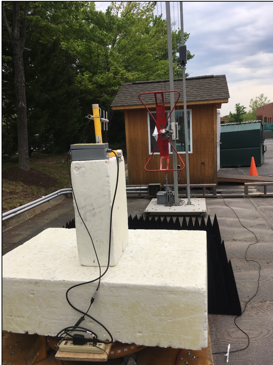
Photograph 8: Yagi Antenna - Back View (Above 1 GHz)
