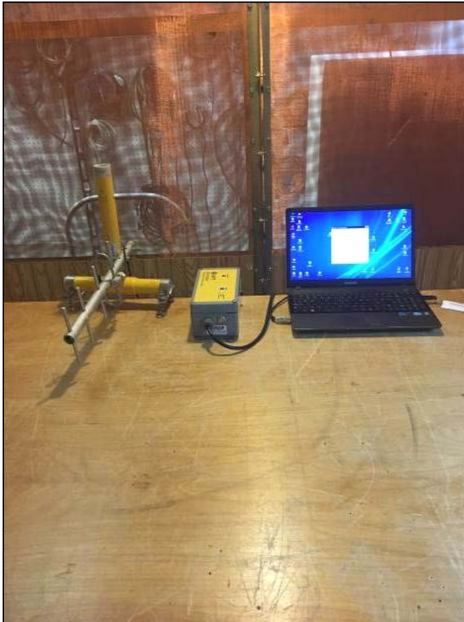
Photograph 11: AC Conducted Emissions - Yagi Antenna - Front View
