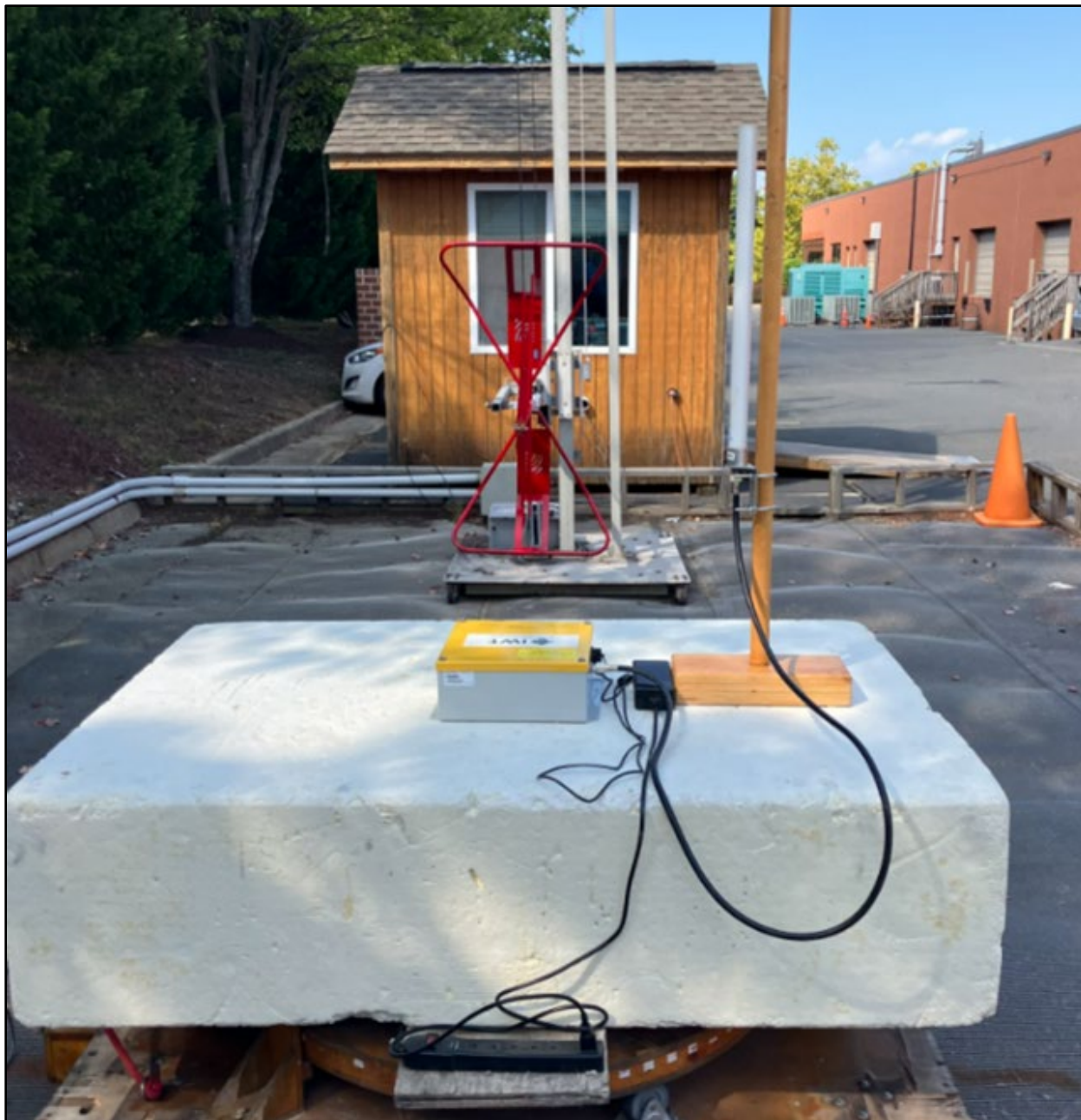
Photograph 6: Collocated Radiated Emissions – Rear View – Omni Antenna
