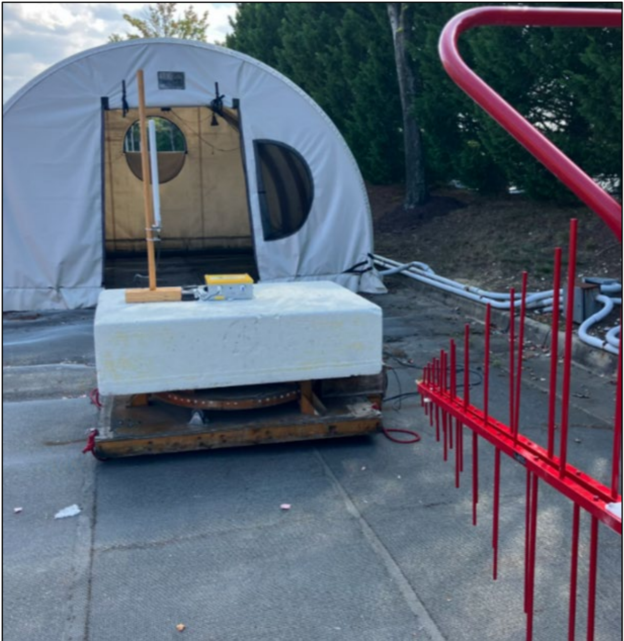
Photograph 5: Collocated Radiated Emissions – Front View – Omni Antenna
