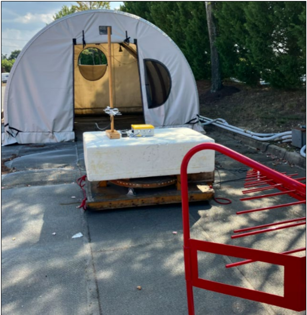
Photograph 3: Collocated Radiated Emissions – Front View – Yagi Antenna
