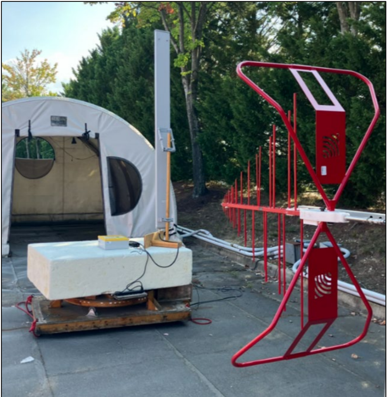
Photograph 2: Collocated Radiated Emissions – Rear View – Sector Antenna
