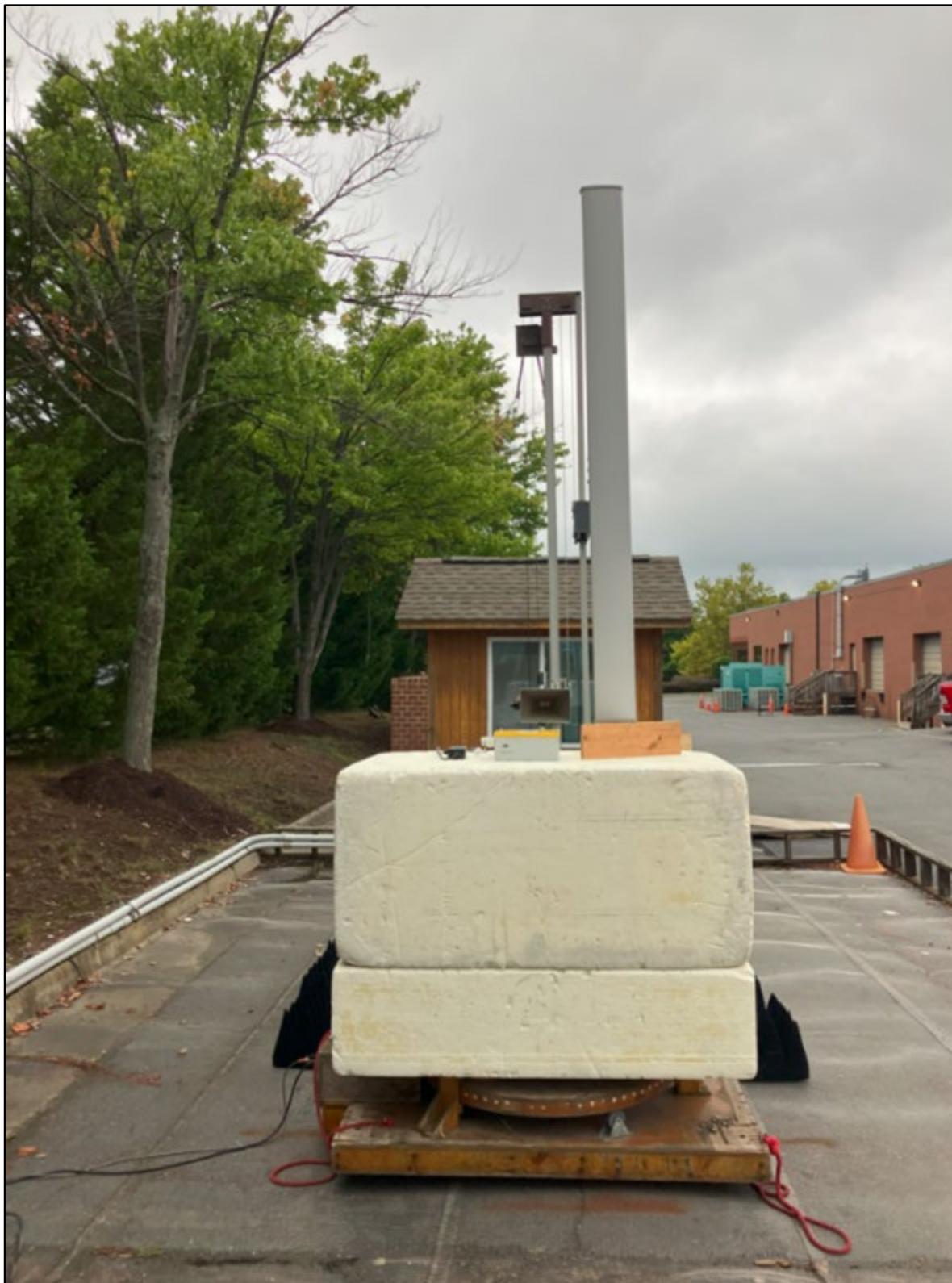
Photograph 9: Radiated Emissions – Front View – Sector Antenna Greater Than 1 GHz – GWN
