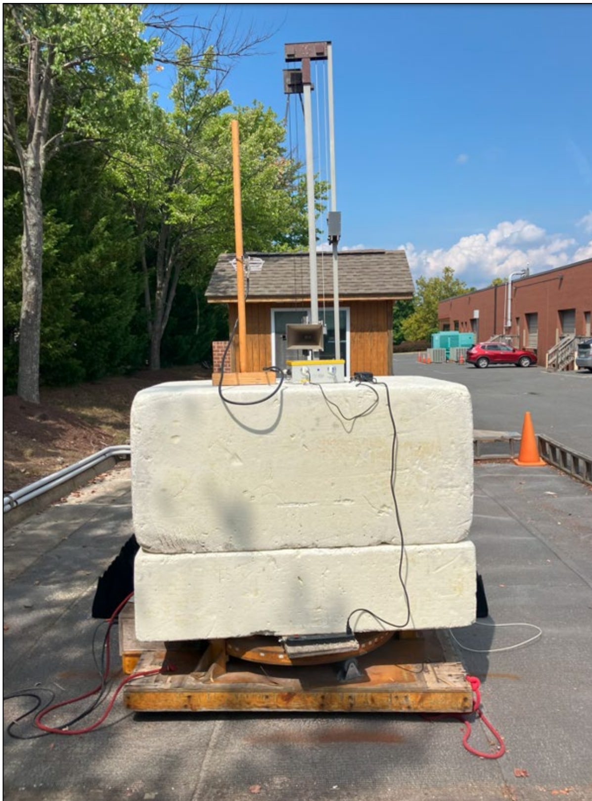
Photograph 2: Radiated Emissions – Rear View – Yagi Antenna Greater Than 1 GHz
