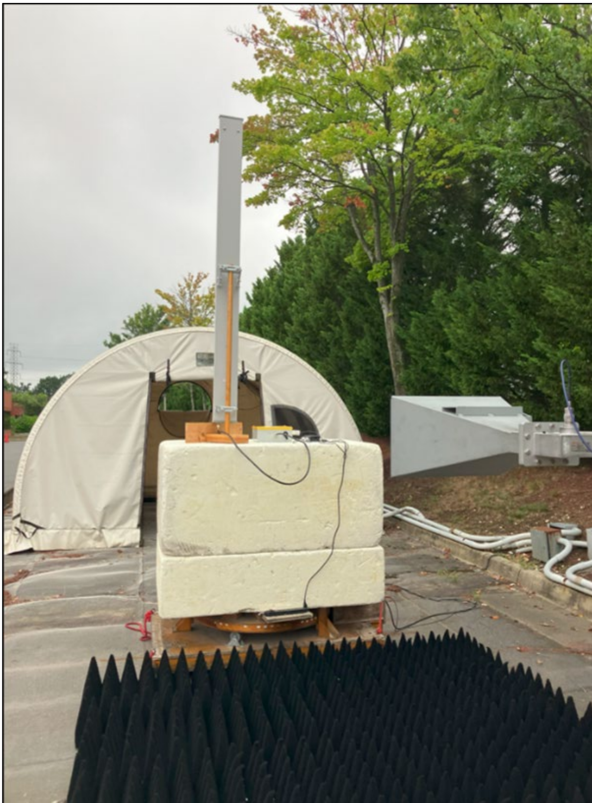
Photograph 10: Radiated Emissions – Rear View – Sector Antenna Greater Than 1 GHz – GWN
