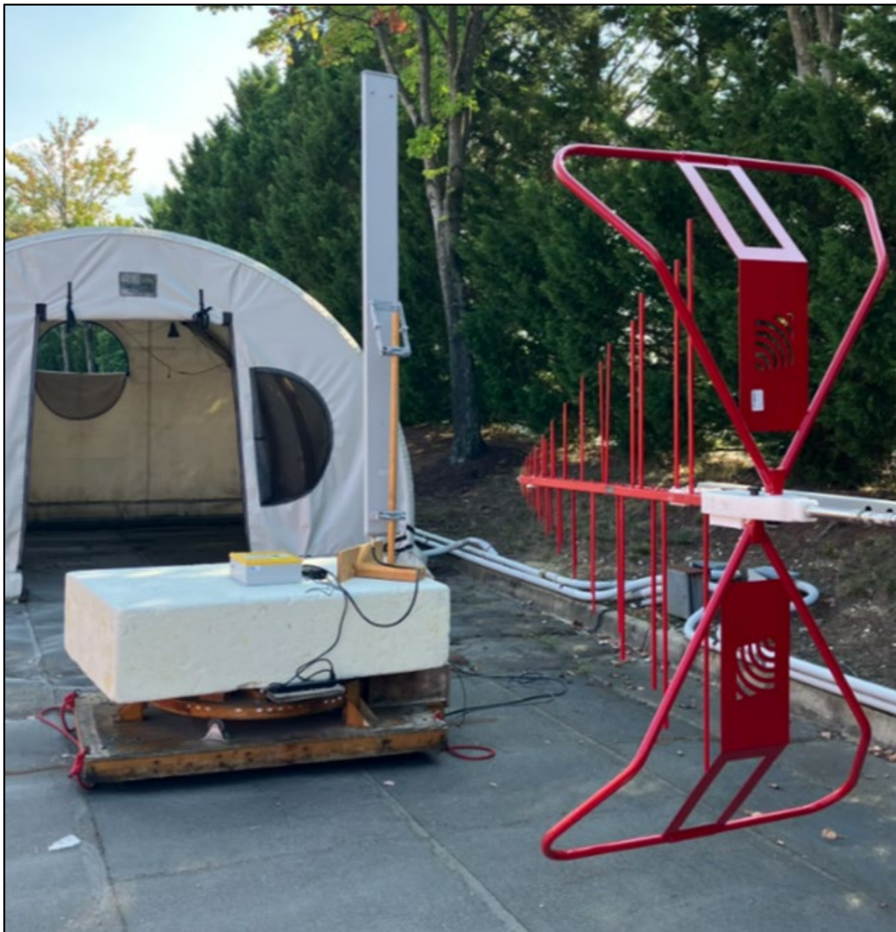
Photograph 14: Radiated Emissions – Rear View – Sector Antenna Less Than 1 GHz– GWN
