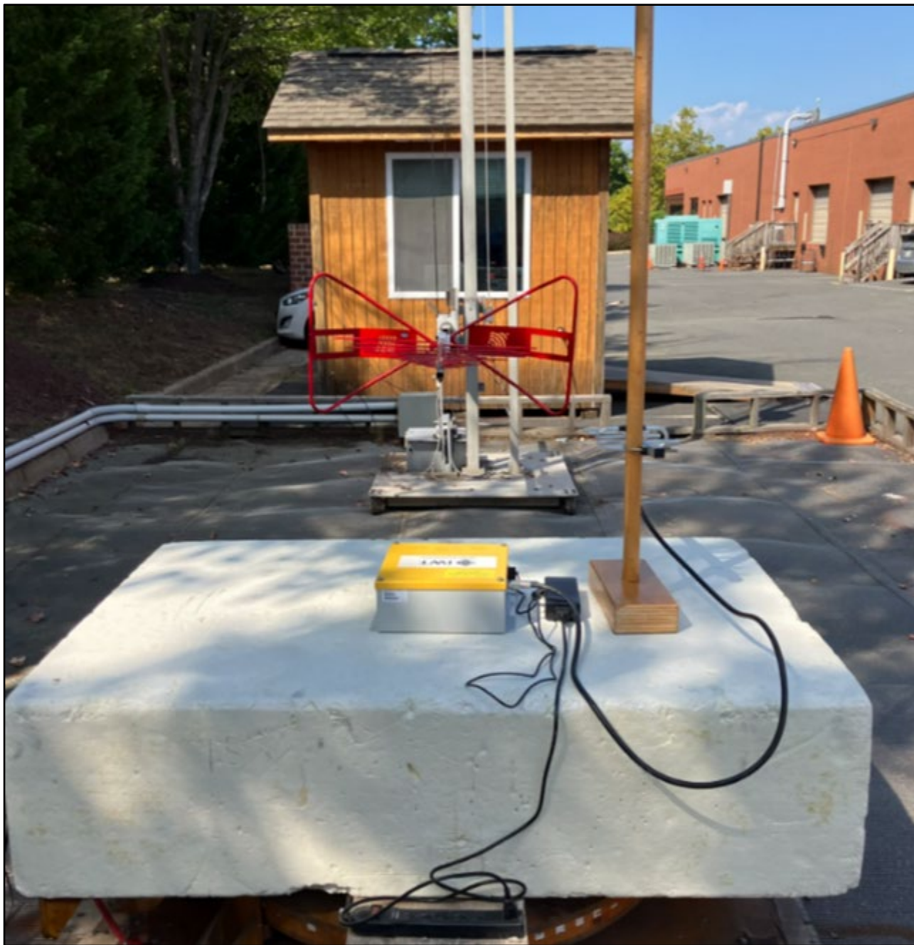
Photograph 4: Radiated Emissions – Rear View – Yagi Antenna Less Than 1 GHz
