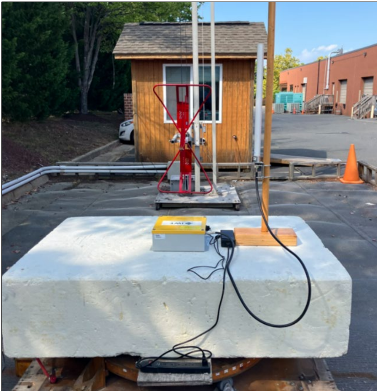
Photograph 8: Radiated Emissions – Rear View – Omni Antenna Less Than 1 GHz
