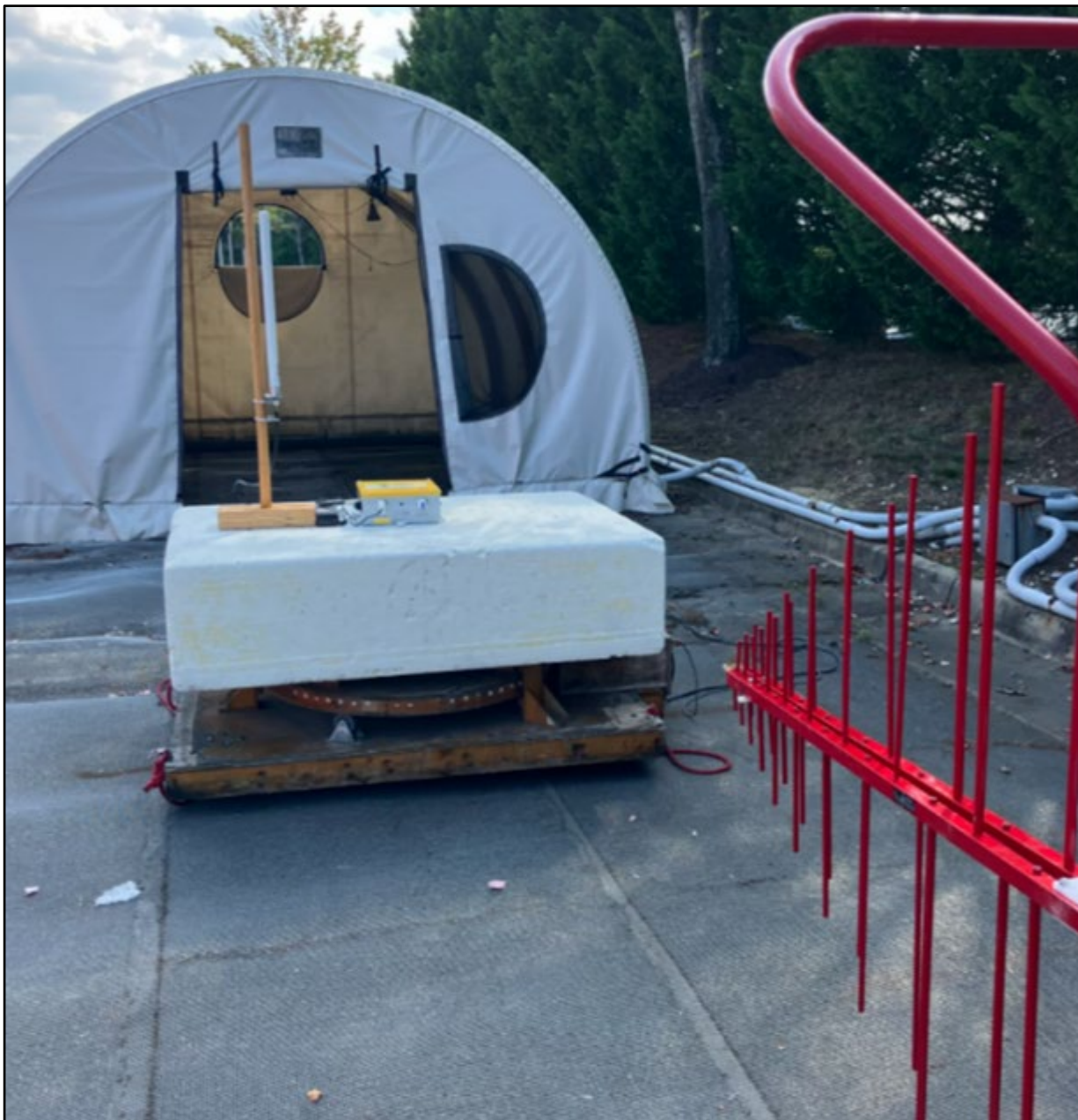
Photograph 7: Radiated Emissions – Front View – Omni Antenna Less Than 1 GHz
