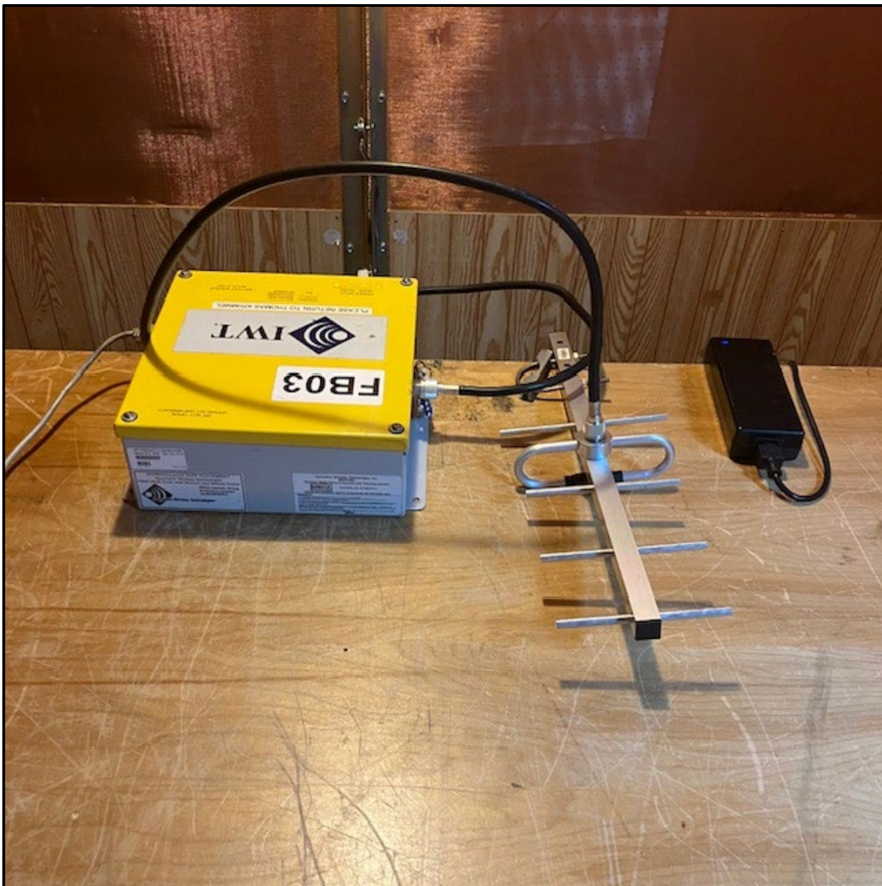
Photograph 20: Conducted Line Emissions – Front View – FMN
