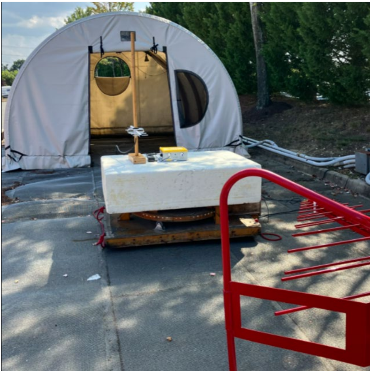
Photograph 3: Radiated Emissions – Front View – Yagi Antenna Less Than 1 GHz
