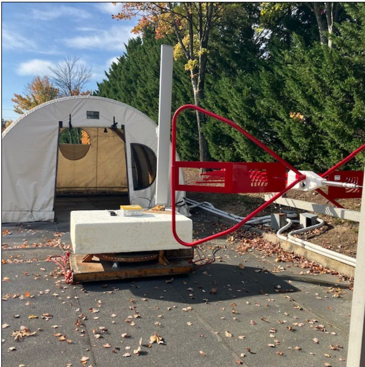
Photograph 15: Radiated Emissions – Front View – Sector Antenna Less Than 1 GHz – FMN
