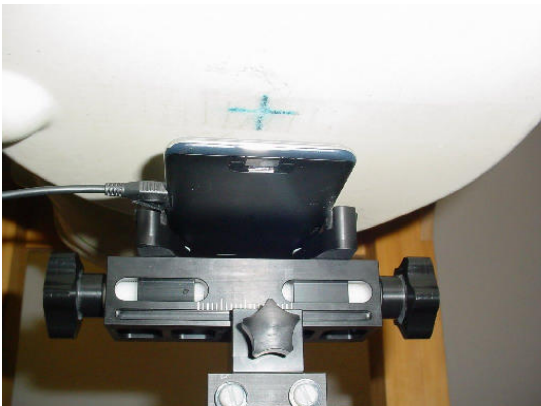
Photo 20: Test position body worn front side (15 mm distance)
