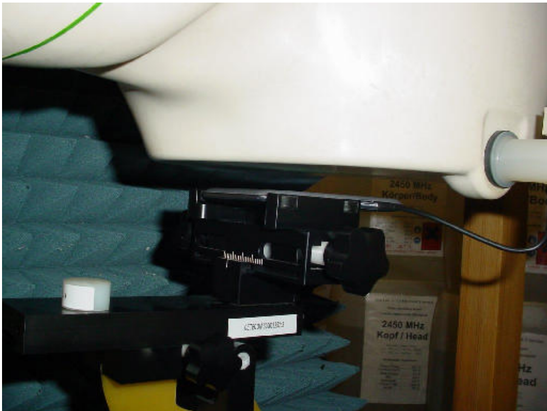
Photo 20: Test position body worn front side (15 mm distance)
