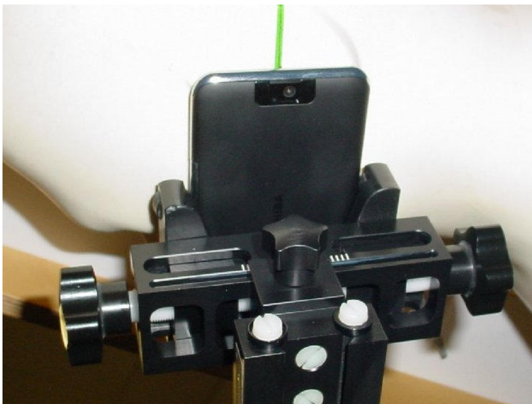
Photo 12: Test position left hand tilted 15°
