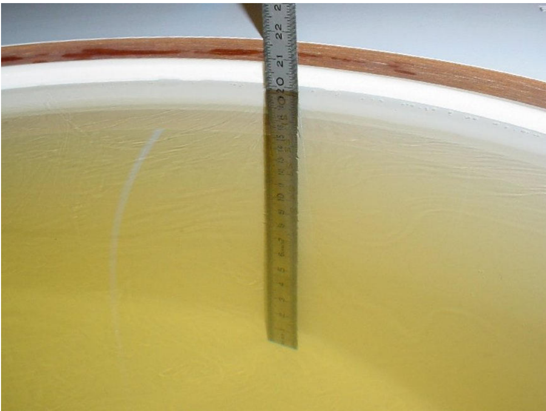
Photo 24: Liquid depth 850 MHz body simulating liquid
