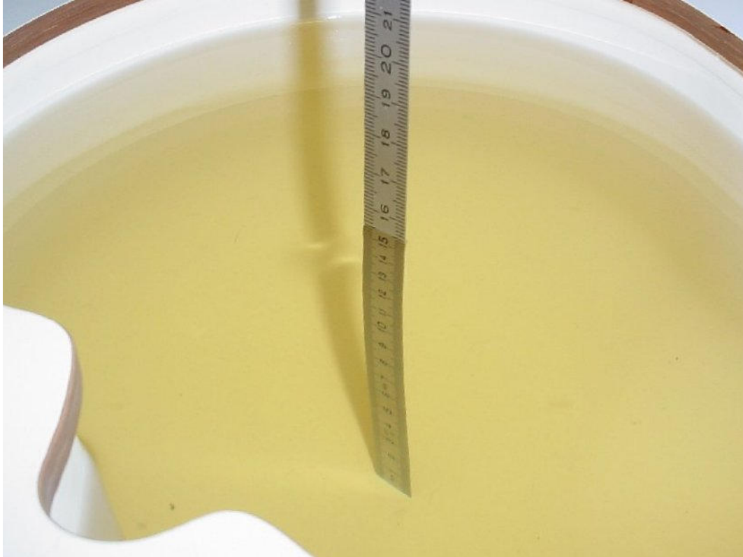
Photo 24: Liquid depth 850 MHz body simulating liquid
