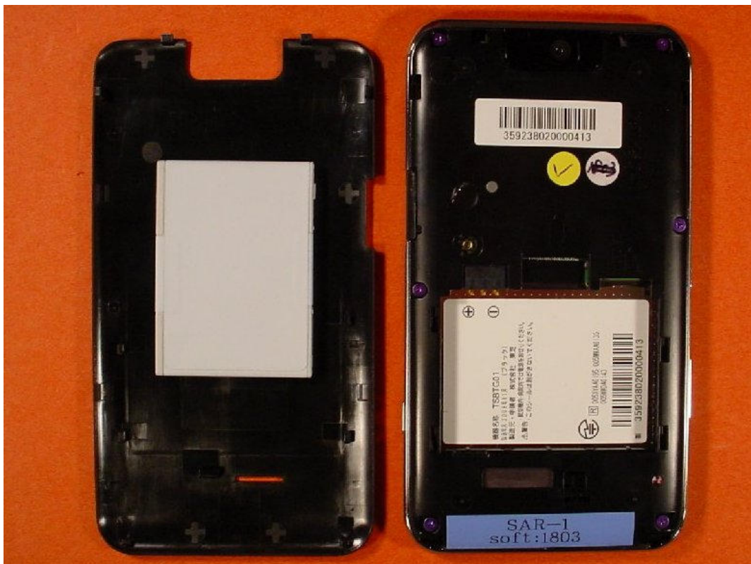
Photo 6: DUT - rear view (open) without battery
