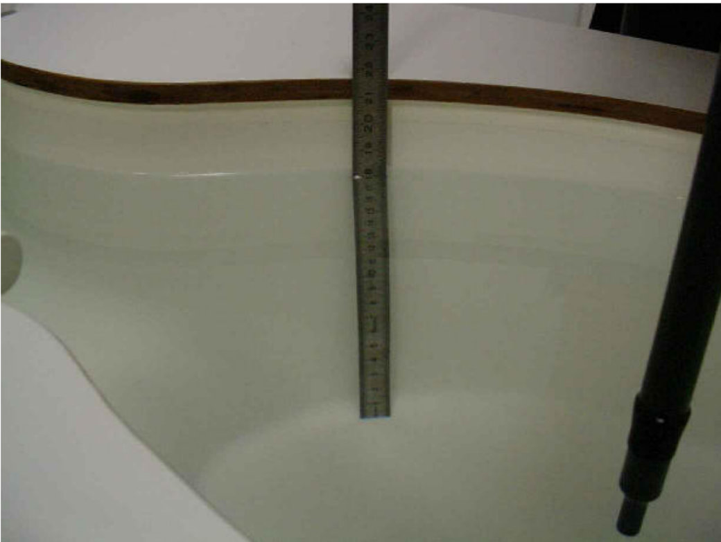
Photo 28: Liquid depth 2450 MHz body simulating liquid
