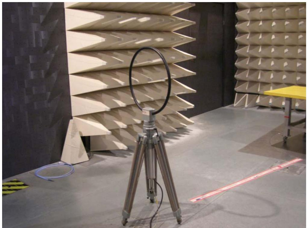
For radiated emissions 30MHz~1GHz
