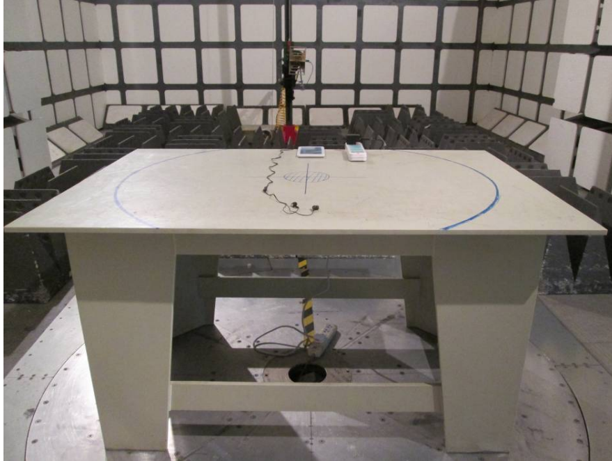
Radiated Emissions – Front View (Above 1 GHz)
