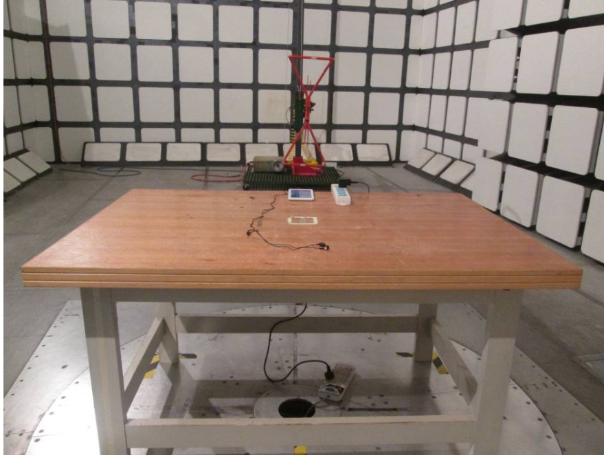
Radiated Emissions – Front View (Below 1 GHz)
