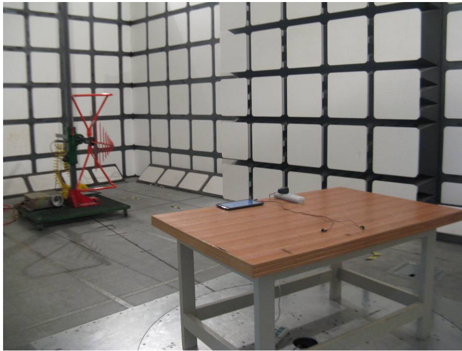
Radiated Emissions - Rear View (charging & multimedia playing)
