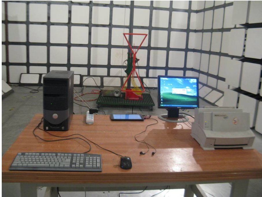
Radiated Emissions - Rear View (charging & downloading)
