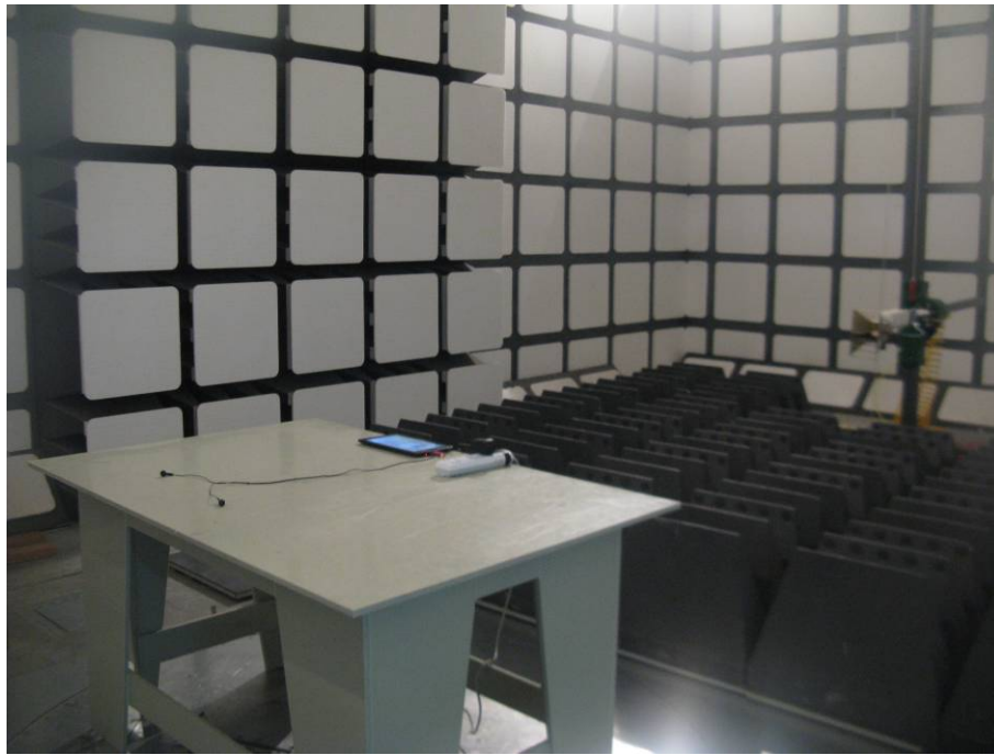
Radiated Emissions - Rear View (charging & multimedia playing)
