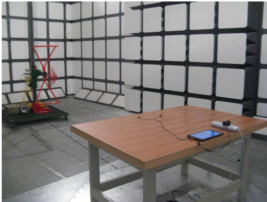
Radiated Emissions - Rear View (charging & multimedia playing)
