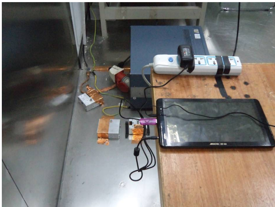
Conduction Emissions - Side View (charging & multimedia playing)
