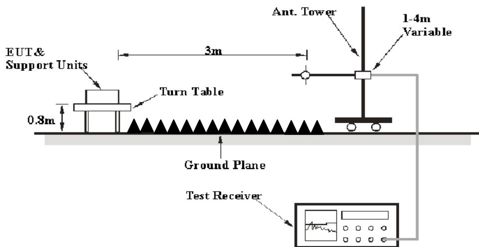
The radiated emission tests were performed in the 3 meters chamber test site, using the setup accordance with the ANSI C63.17 - 2006. The specification used was the FCC 15§ 15.319(g).
