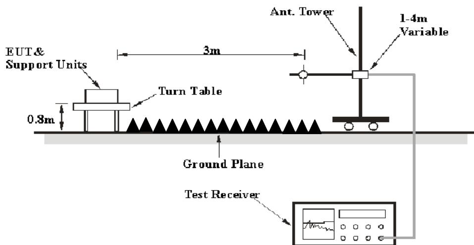
The radiated emission tests were performed in the 3 meters test site, using the setup accordance with the ANSI C63.17 - 2006. The specification used was the FCC 15.209 and FCC 15.319(g) limits.
