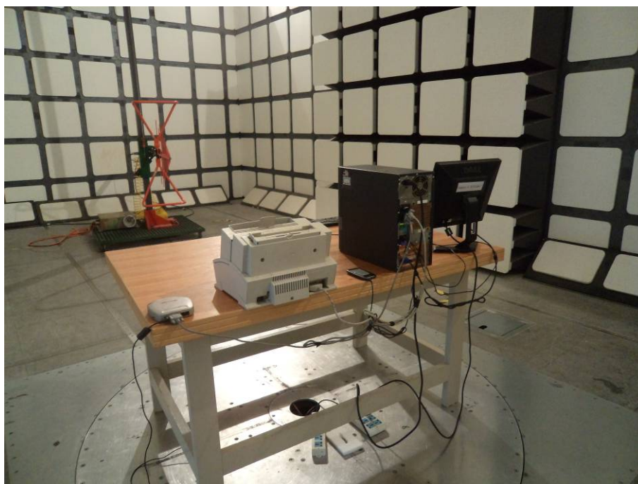
Radiated Emissions - Rear View (Downloading mode)
