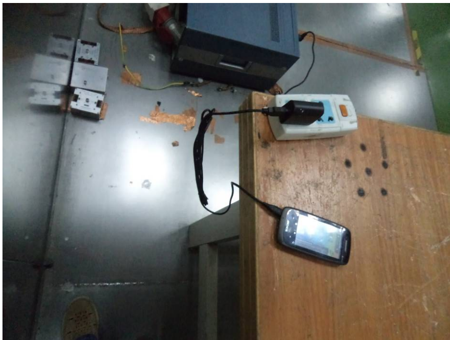
Conduction Emissions - Side View (Charging & Media Playing)
