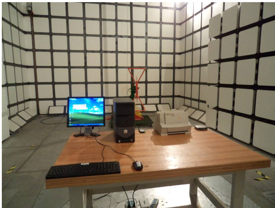
Radiated Emissions - Front View (Downloading mode)
