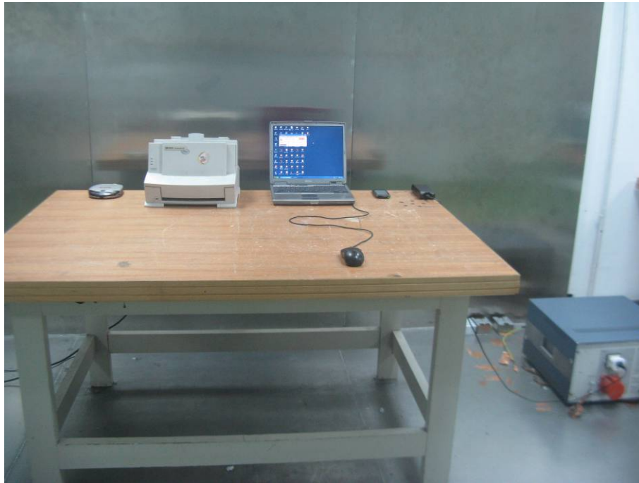
Conduction Emissions - Front View (Downloading mode)
