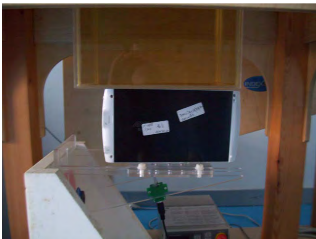
Fig.4 EUT Position 2(against the bottom)
