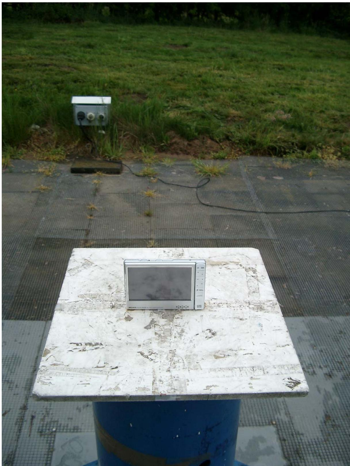
Test Setup Photos : Conducted emissions AC Port
