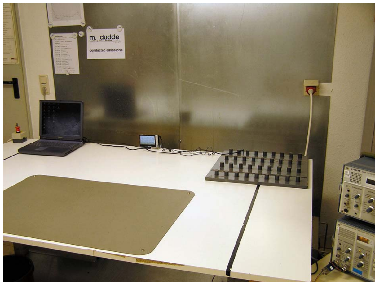
Test Setup Photos : Conducted emissions AC Port
