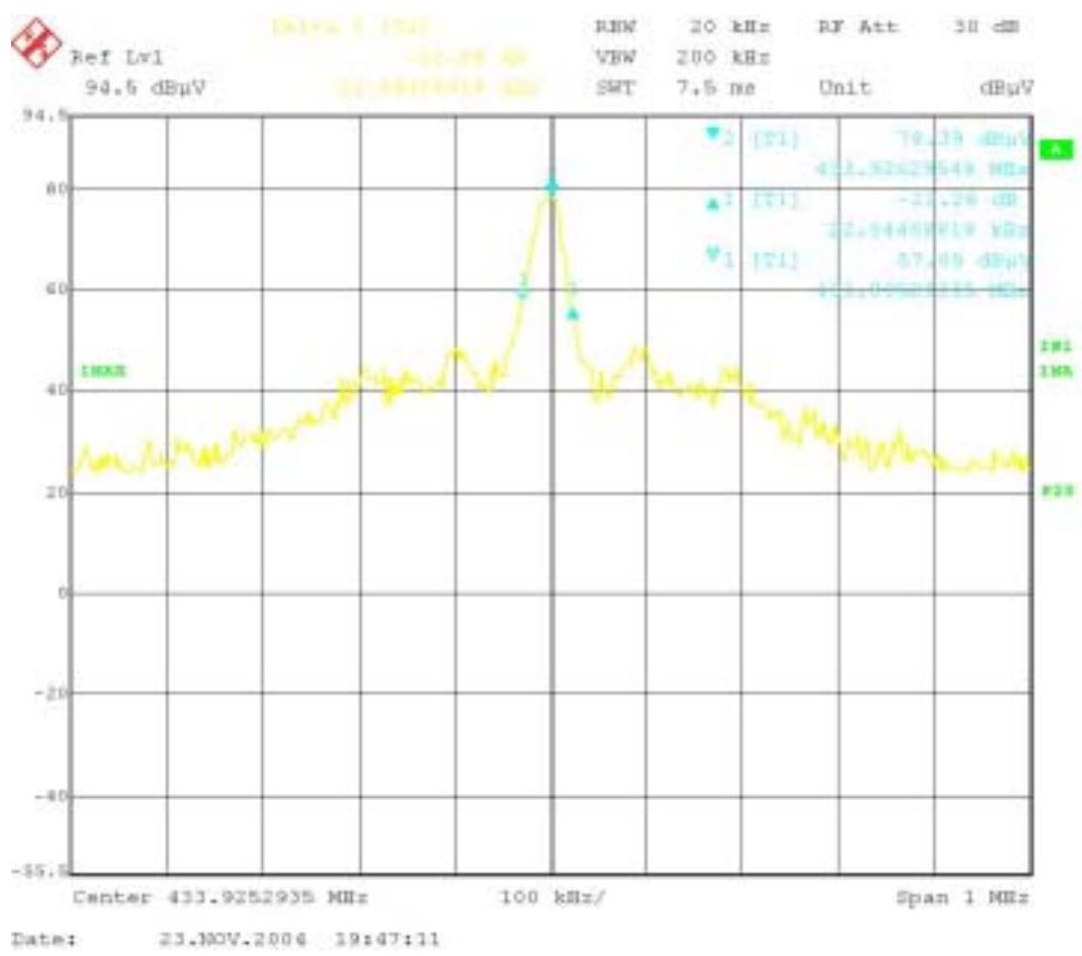
Measured bandwidth is 53.103 KHz < 433.92 MHz  $\times$  0.25% = 1.0848 MHz
