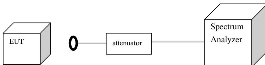
Remark: the attenuator is the built-in part of spectrum analyzer.
