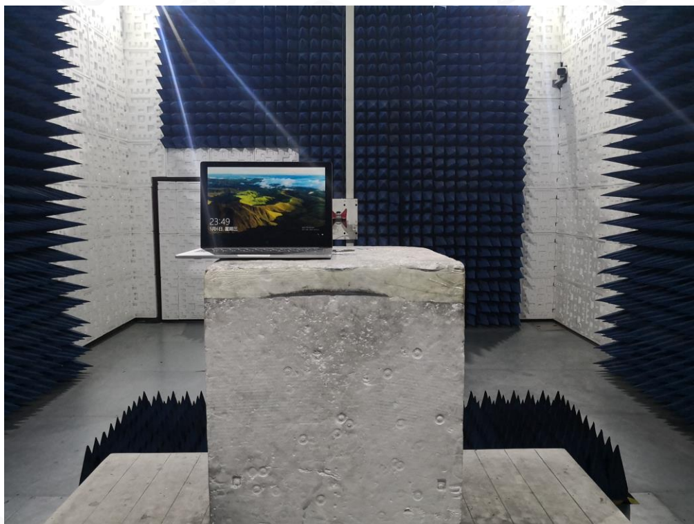
RADIATED EMISSION TEST SETUP ABOVE 1GHZ
