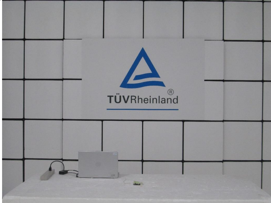
Photograph 1: Test Setup for Spurious Emissions (Front View 1)
