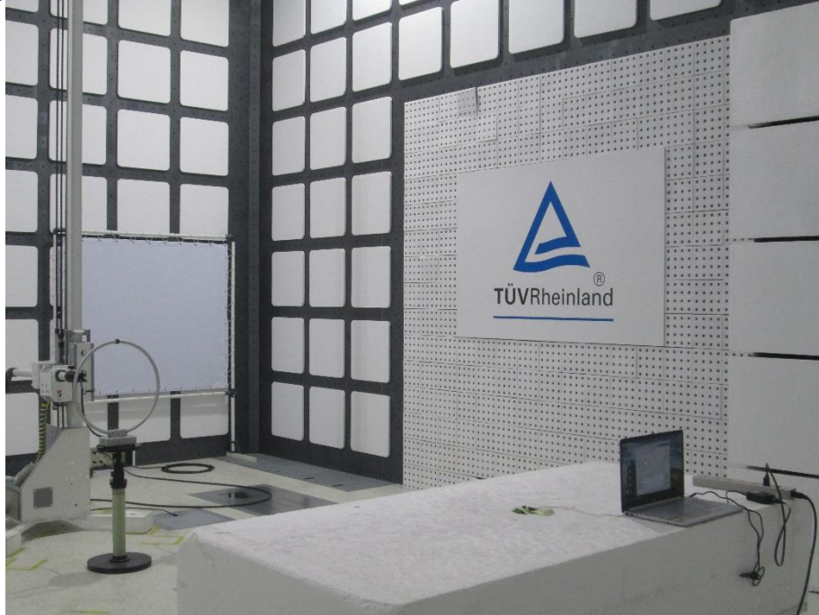
Photograph 3: Test Setup for Spurious Emissions (Back View 1)
