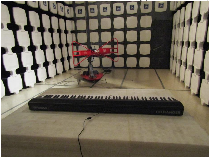
Measurement of Radiated Emission Test Set Up (30MHz to 1000MHz)
