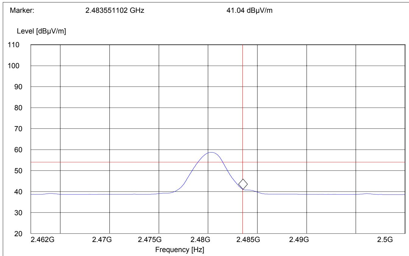
**BAND EDGE COMPLIANCE****§15.247 (c)****High frequency section (spurious in the restricted band 2483.5 – 2500 MHz)****Peak Measurement****(This plot is valid for both Hopping ON & OFF)**
