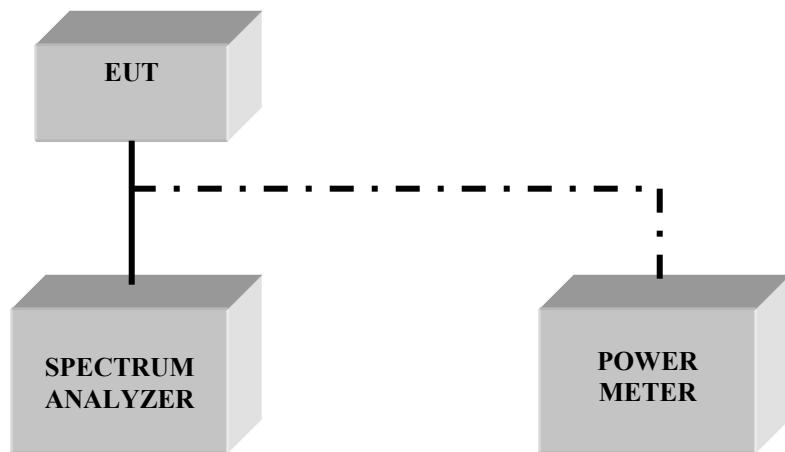
**Radiated Testing****ANECHOIC CHAMBER**
