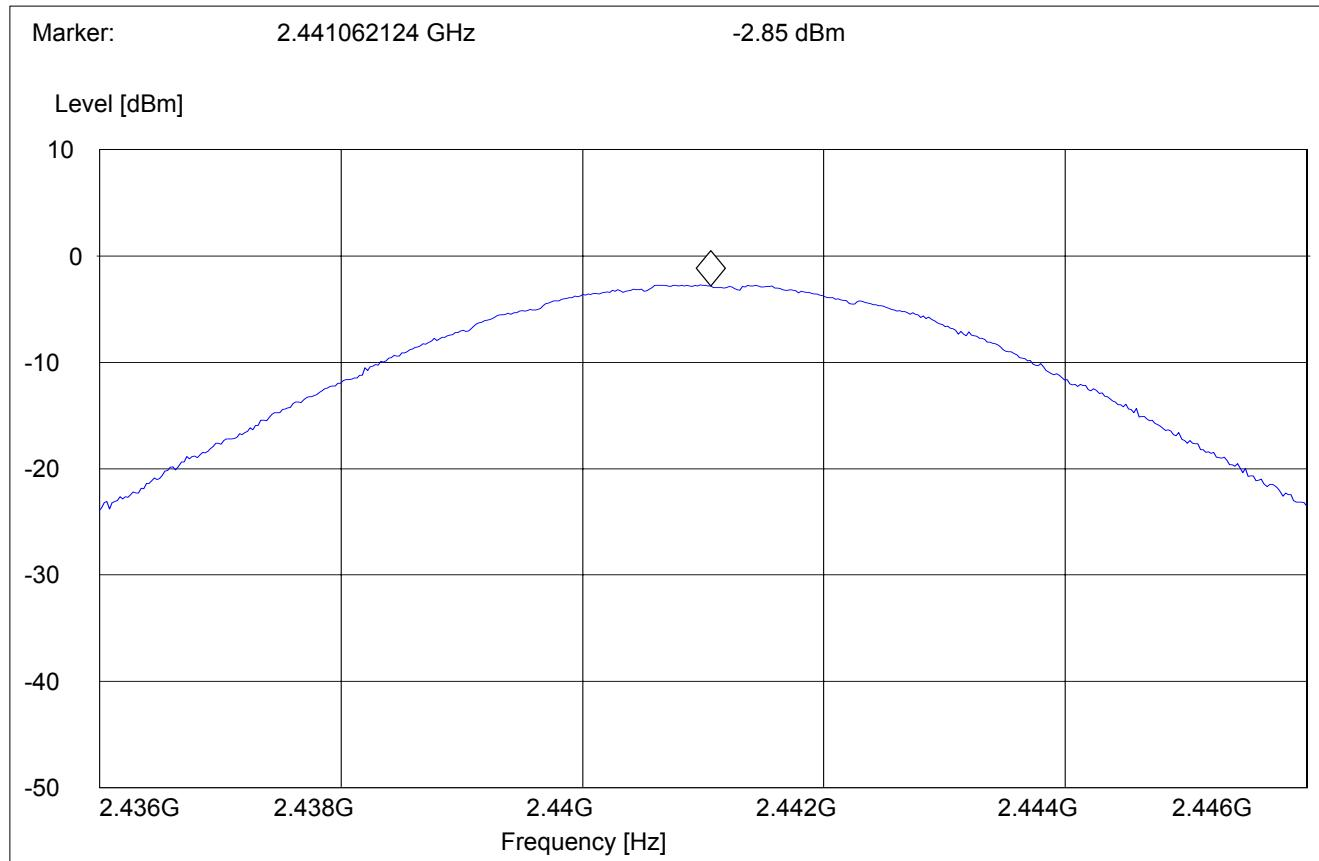
**PEAK OUTPUT POWER (RADIATED)****§15.247 (b) (1)****Highest Channel: 2480MHz**
