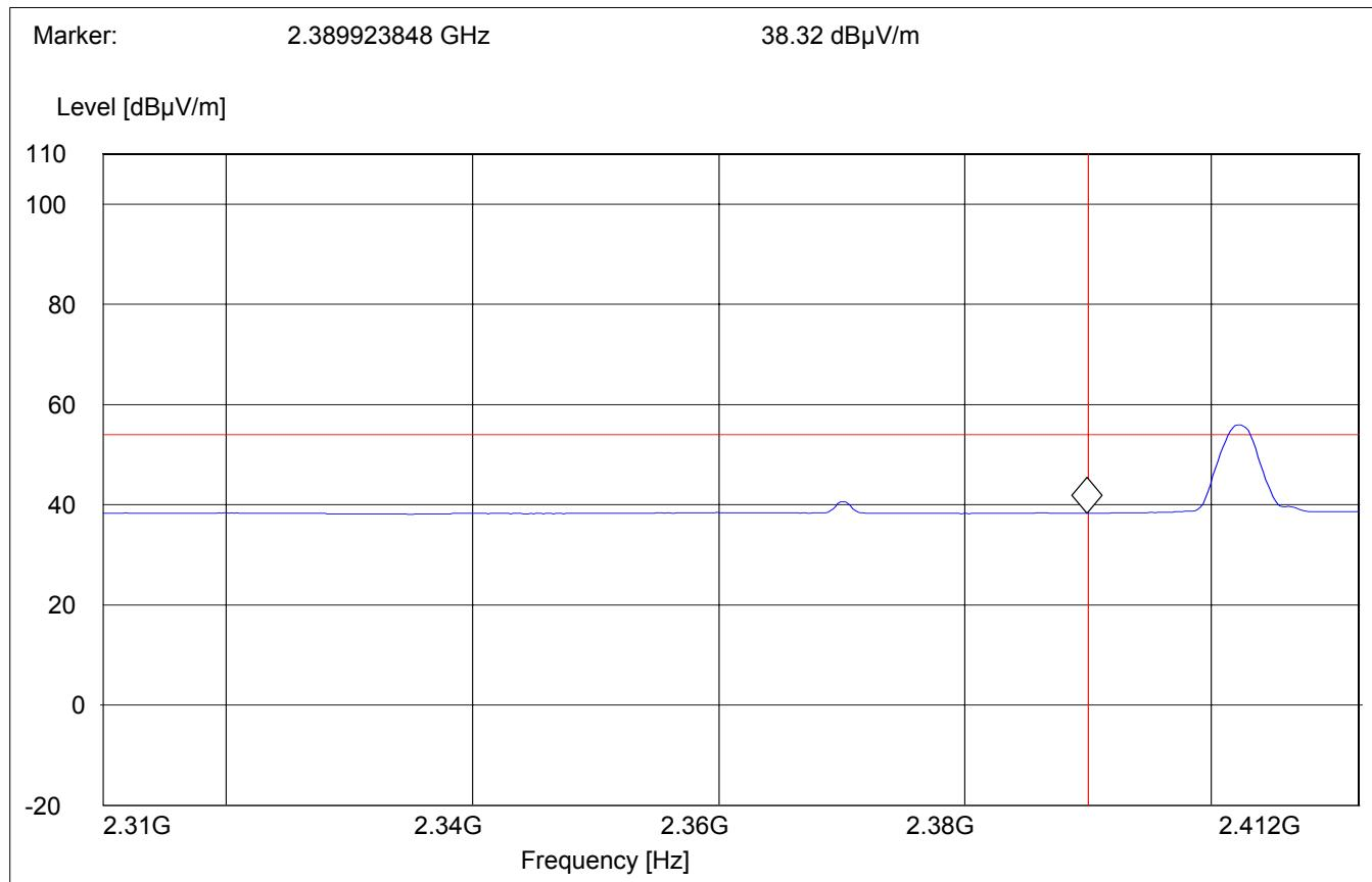
**BAND EDGE COMPLIANCE****§15.247 (c)****Low frequency section (spurious in the restricted band 2310 – 2390 MHz)****Peak Measurement****(This plot is valid for both Hopping ON & OFF)**
