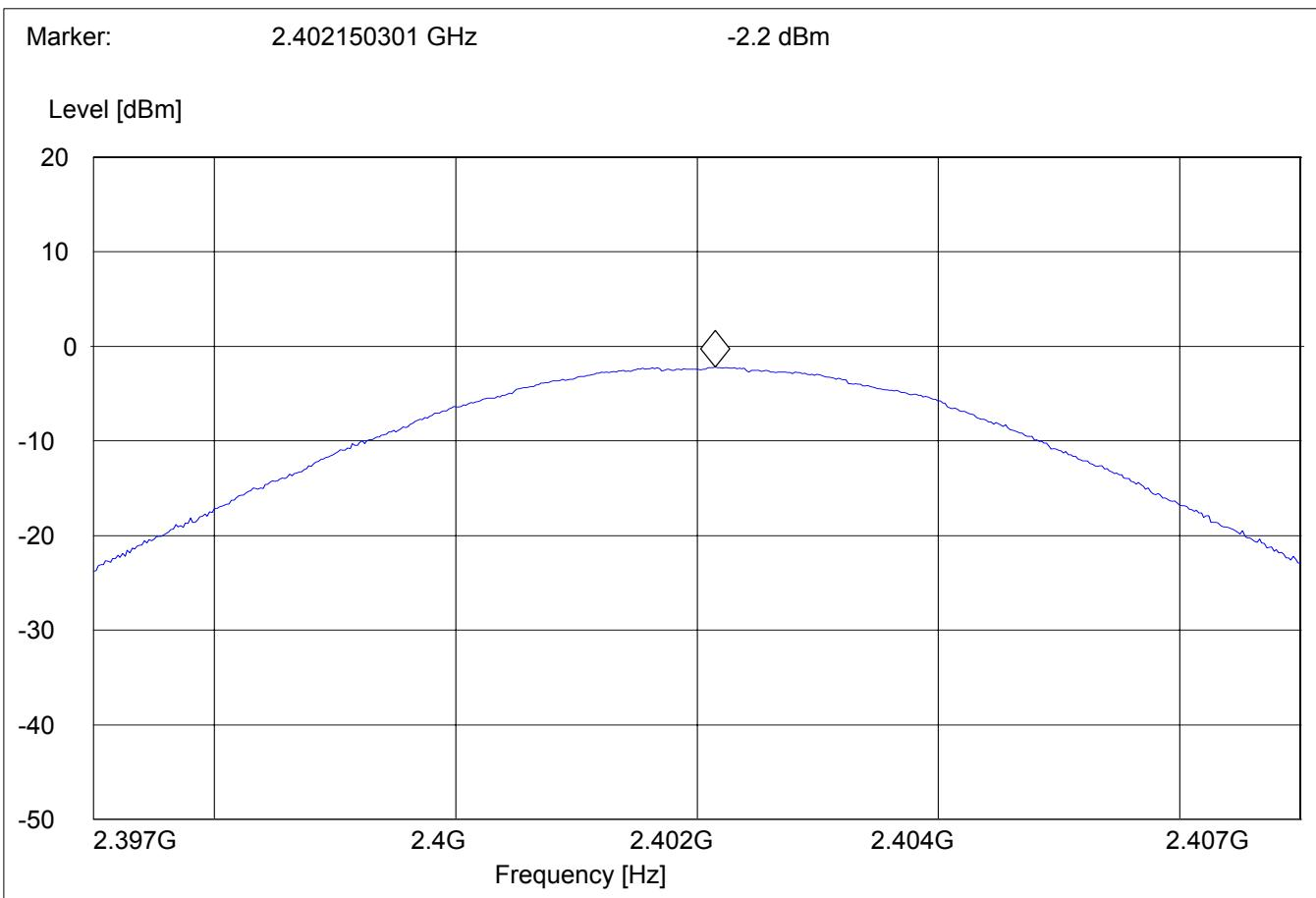
**PEAK OUTPUT POWER (RADIATED)****§15.247 (b) (1)****Mid Channel: 2441MHz**
