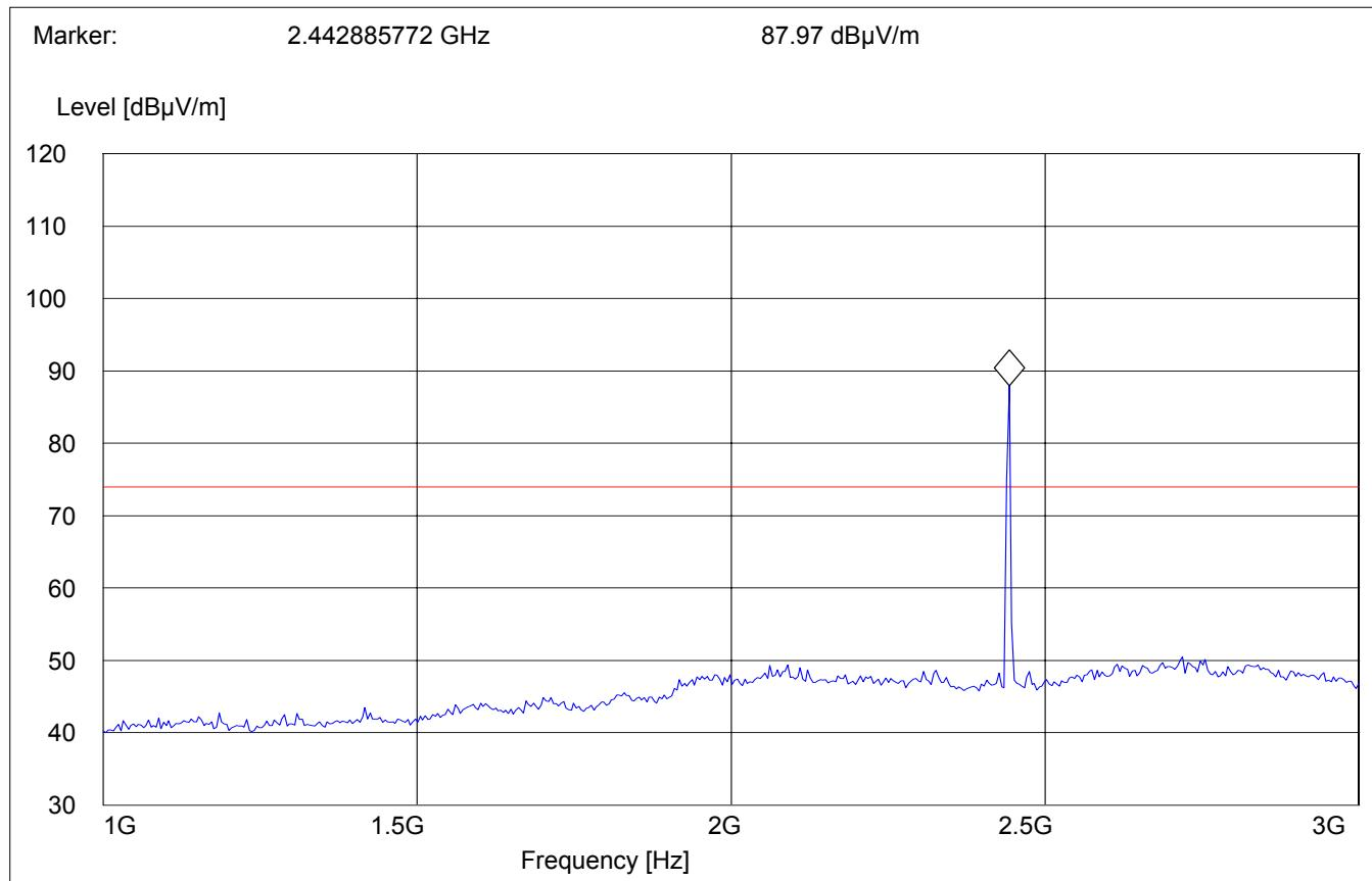
**EMISSION LIMITATIONS - Radiated (Transmitter)****§ 15.247 (c) (1)****Middle Channel (2441MHz): 3GHz – 18GHz****Average**
