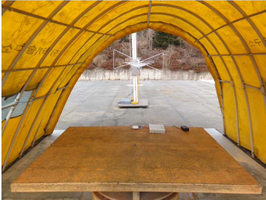
Photograph 2 : Setup for radiated Emissions (above 30 MHz)
