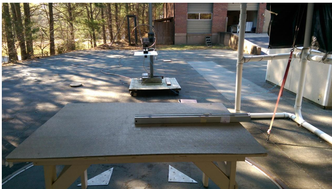
Figure 3. Radiated Emissions Test Setup, .15 MHz to 30 MHz, Back
