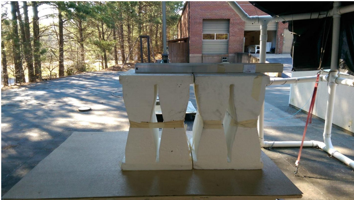
Figure 6. Radiated Emissions Test Setup, above 1 GHz, Back
