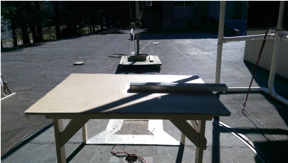
Figure 5. Radiated Emissions Test Setup, 200 MHz to 1GHz, Back
