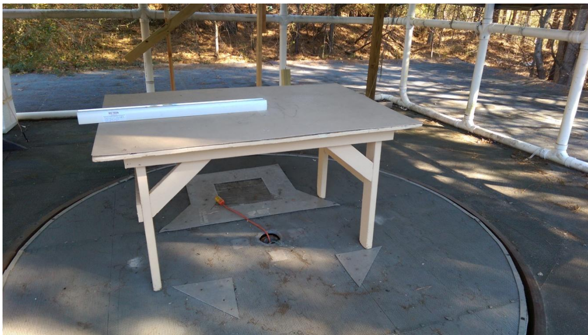
Figure 1. Radiated Emissions Test Setup, Front Below 1 GHz
