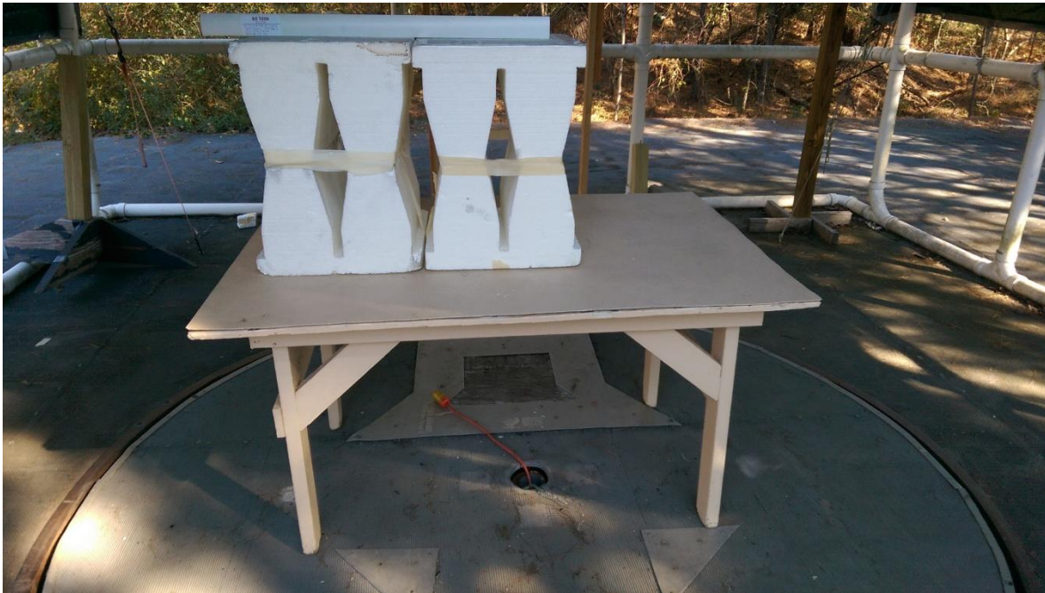
Figure 2. Radiated Emissions Test Setup, Front Above 1 GHz
