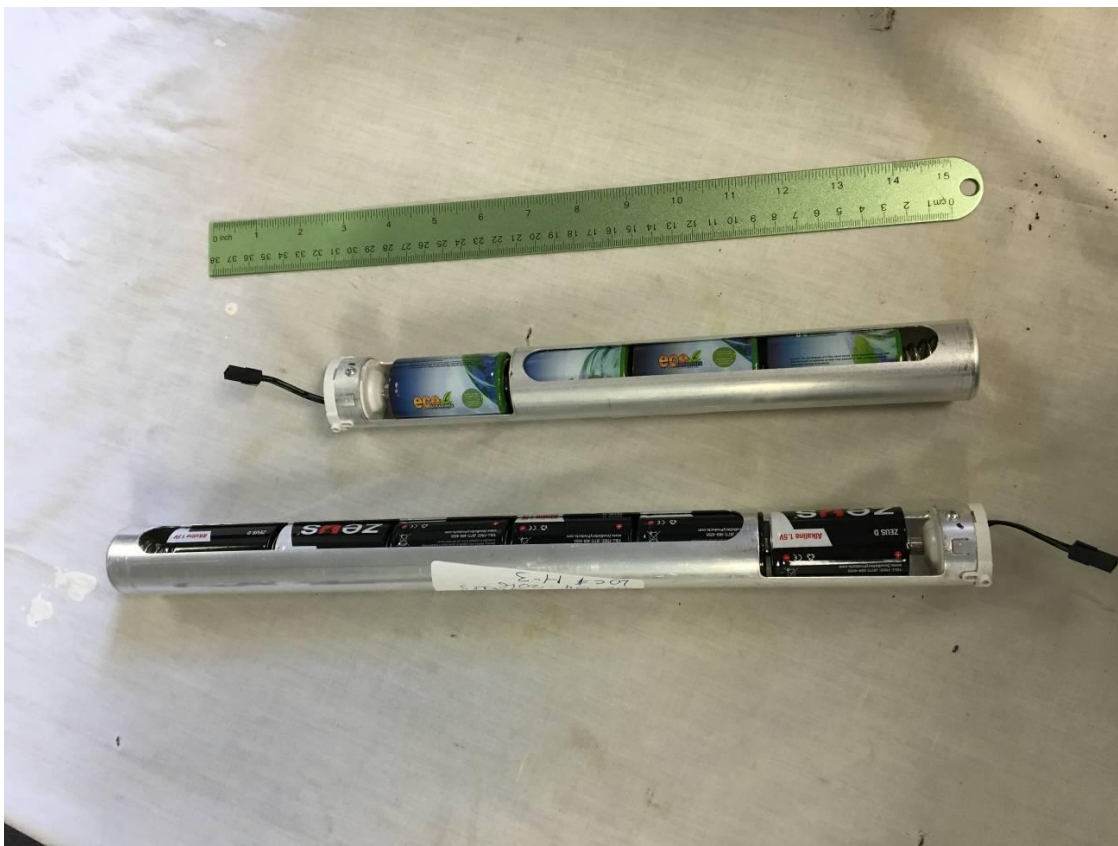
Figure 3. 4 Cell and 6 Cell Battery Pack
