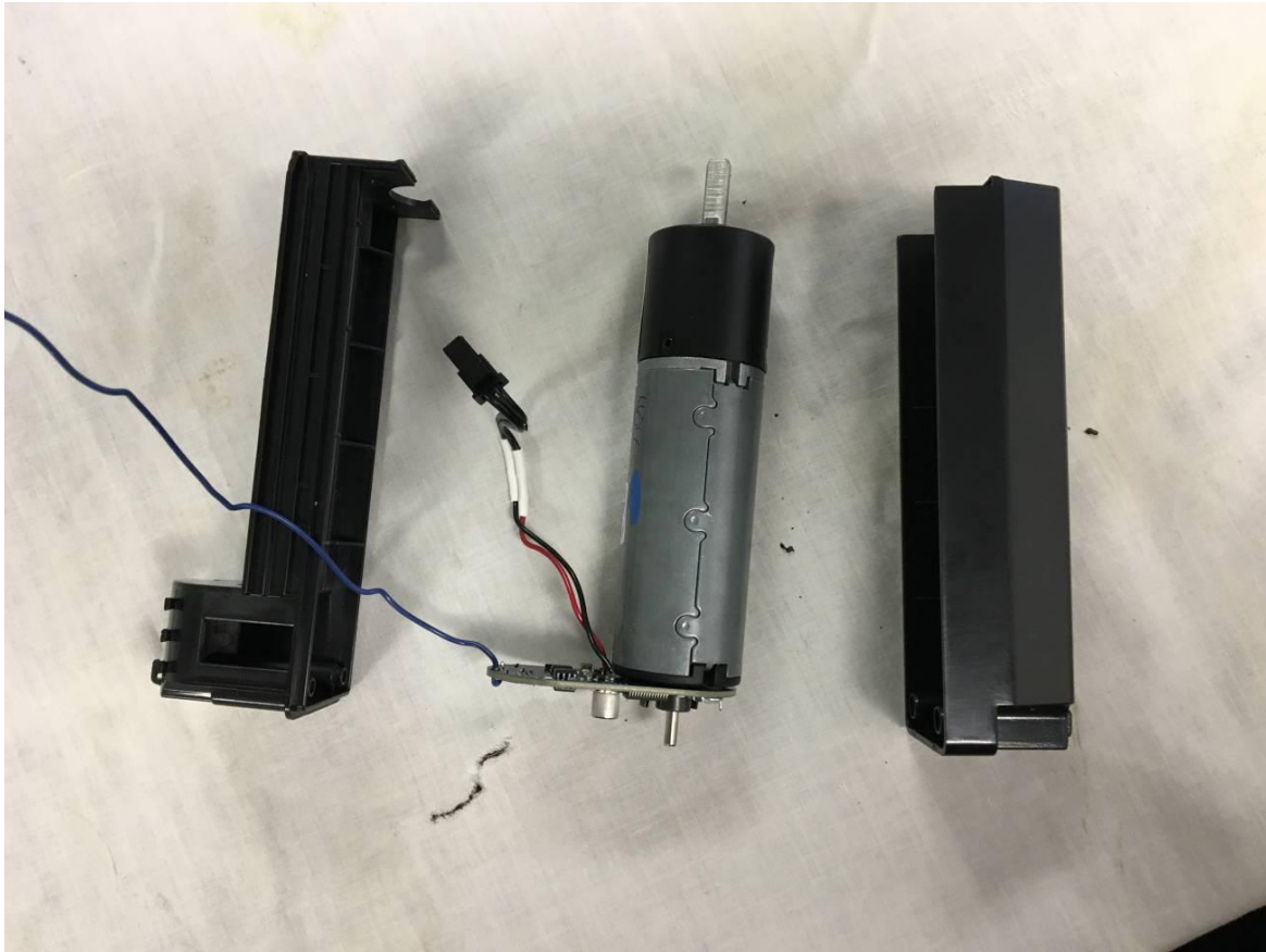
Figure 8. Motor Enclosure Open
