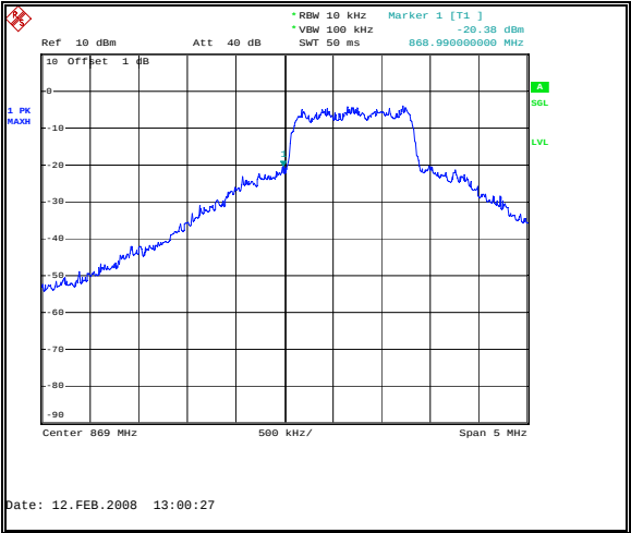
Figure 73: Band-Edge Downlink CDMA Low Channel
