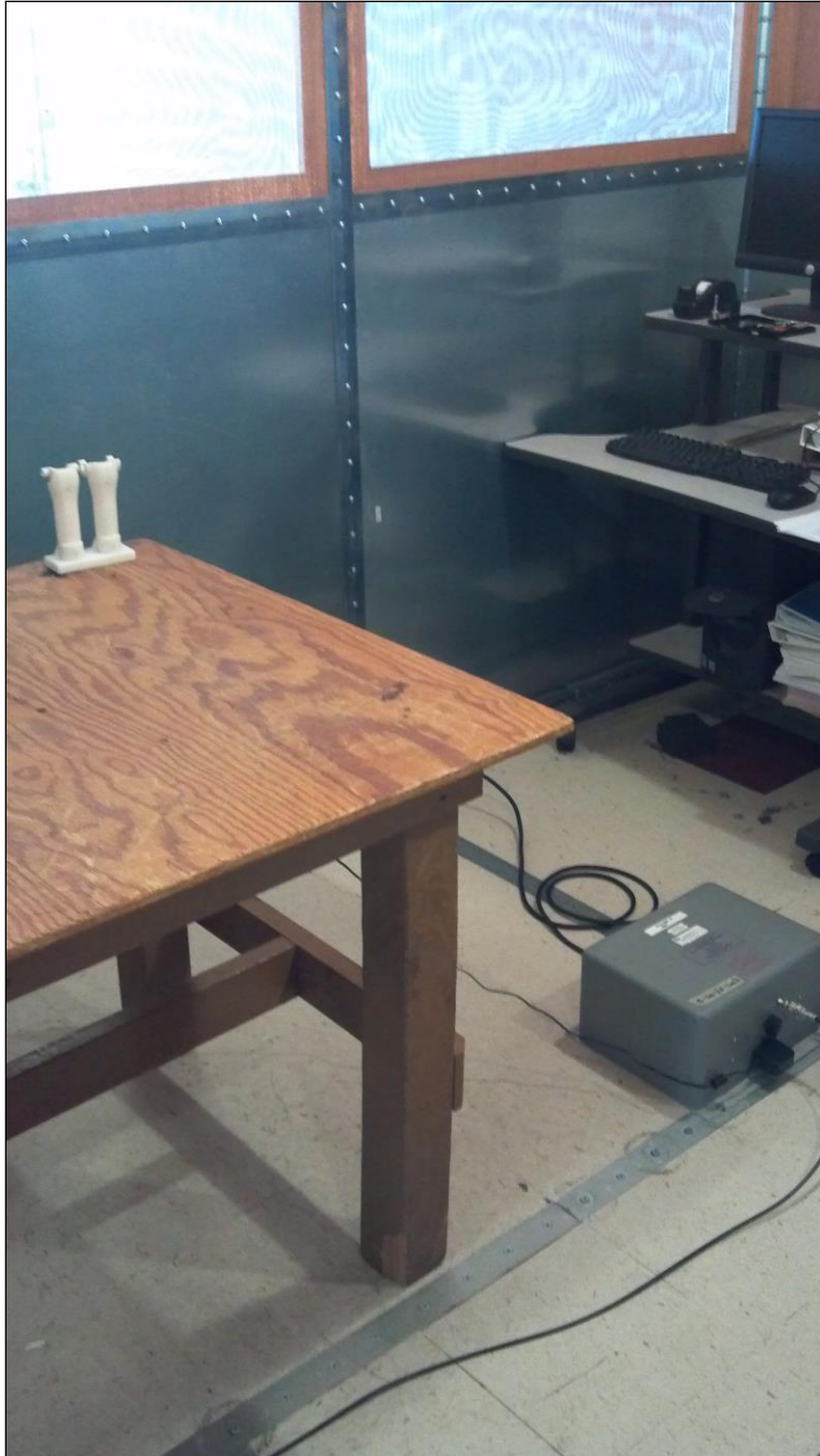
Photograph 1. Conducted Emissions, Test Setup, Charging Mode
