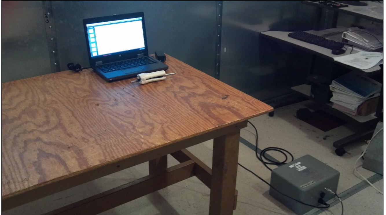
Photograph 2. Conducted Emissions, Test Setup, Transmitting Mode
