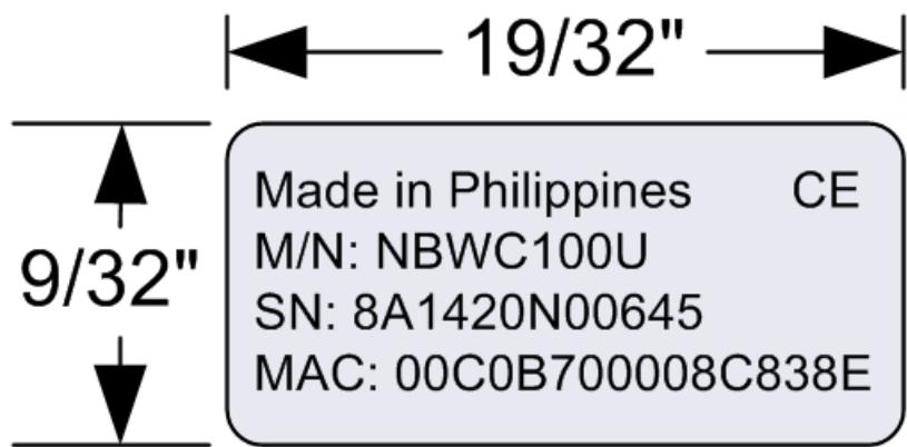
FCC & IC Etching: Location: On Metal Body
