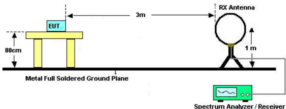
For radiated emission from 30MHz to1GHz
