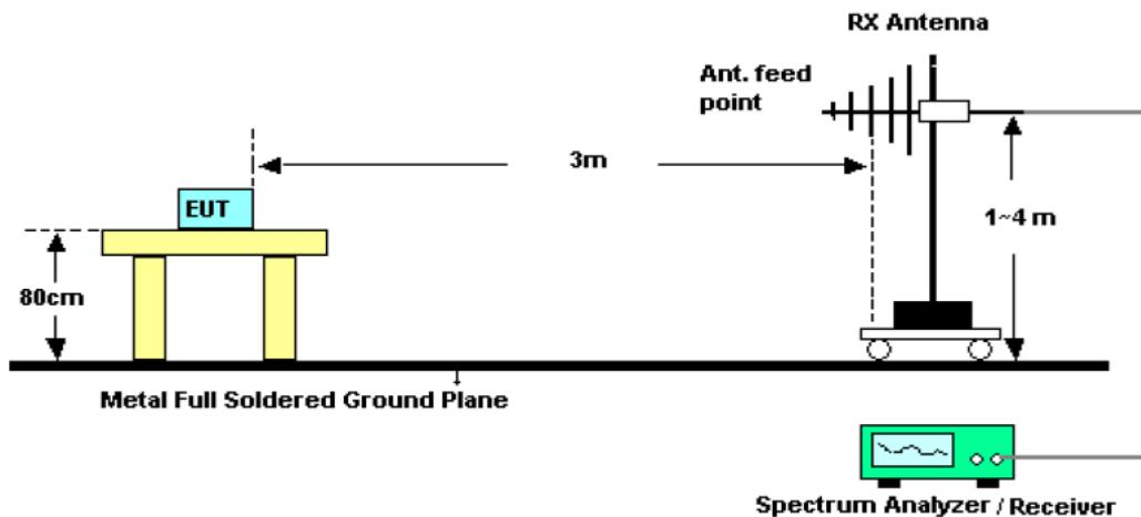
For radiated emission from above1GHz
