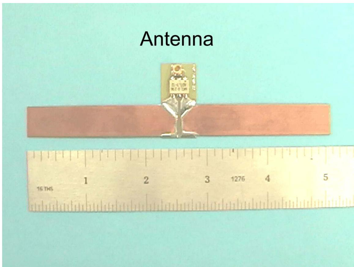
Photo 10 Internal Antenna Close up (Balun)
