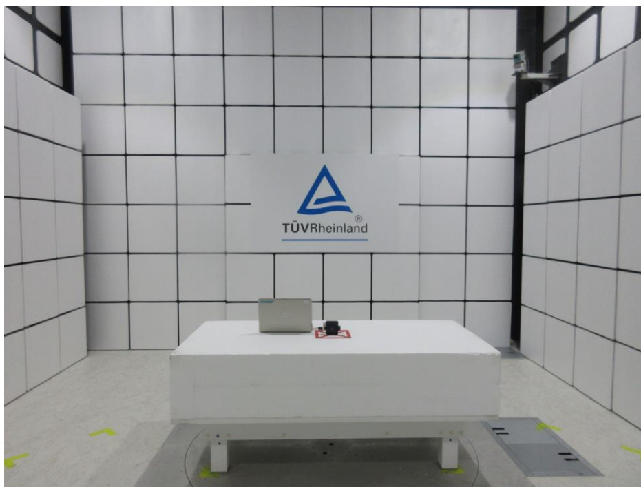
Photograph 1: Set-up for Spurious Emissions (Front View 1)
