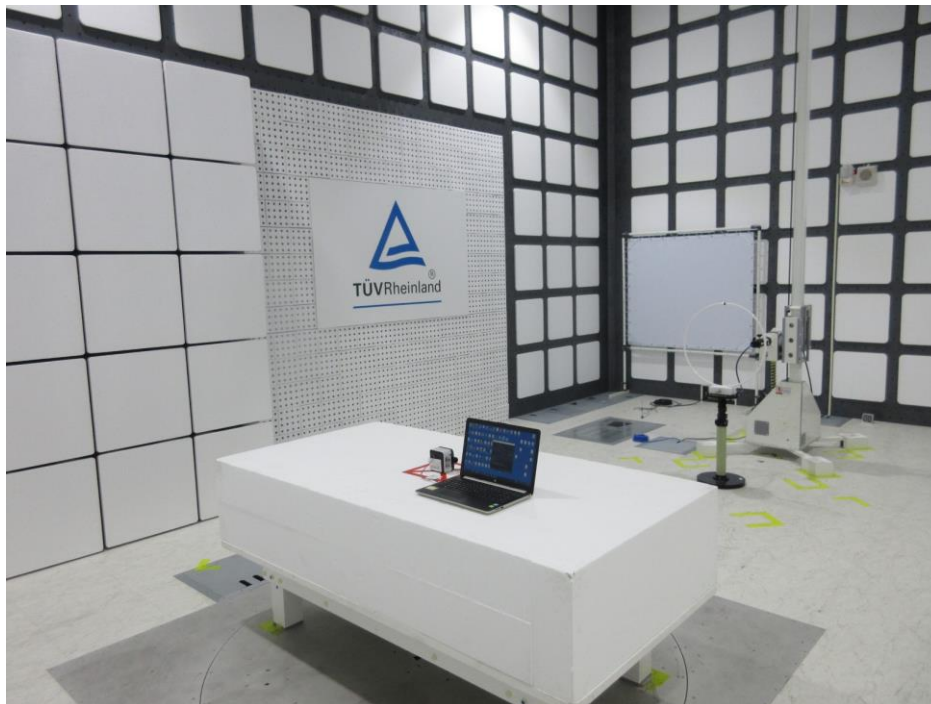
Photograph 5: Set-up for Spurious Emissions (Back View 3)
