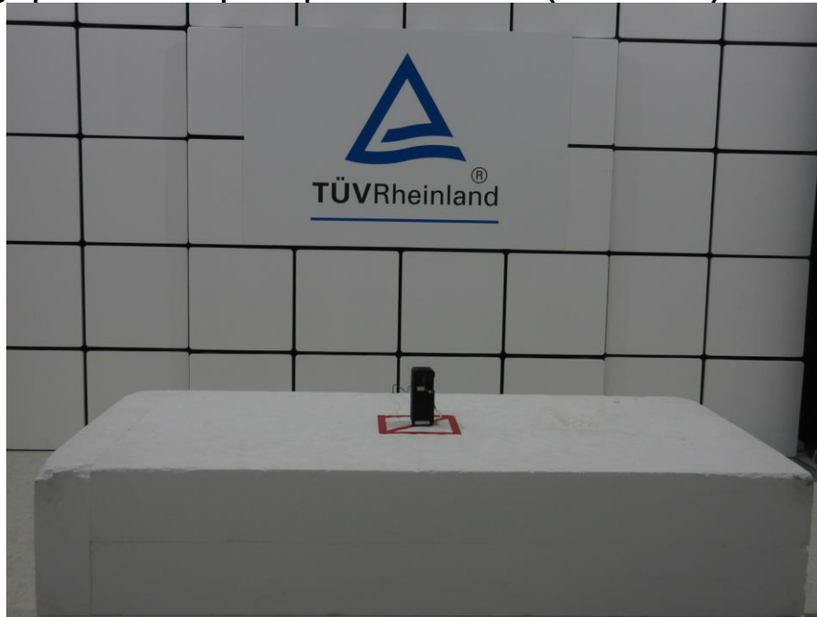
Photograph 2: Test Setup for Spurious Emissions (Front View 2)
