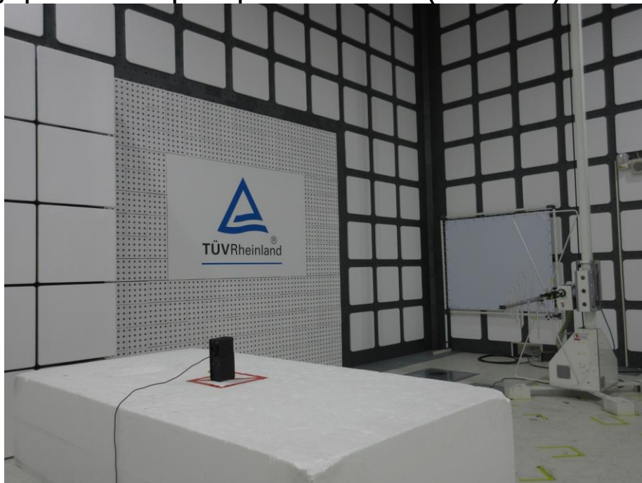
Photograph 6: Test Setup for Spurious Emissions (Back View 4)
