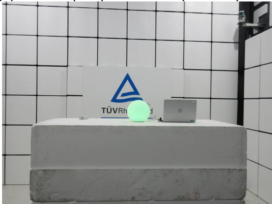
Photograph 2: Test Setup for Spurious Emissions (Front View 2)
