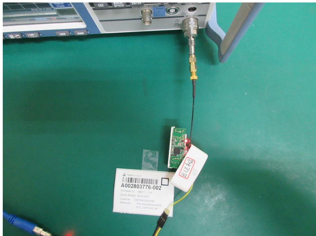
Photograph 8: Set-up for Conducted Testing (View 2)
