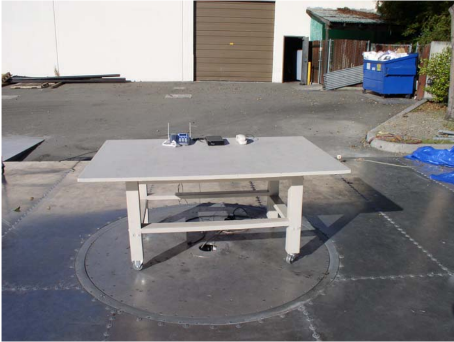
Base Radiated Emission – Front View (2.4GHz FHSS)
