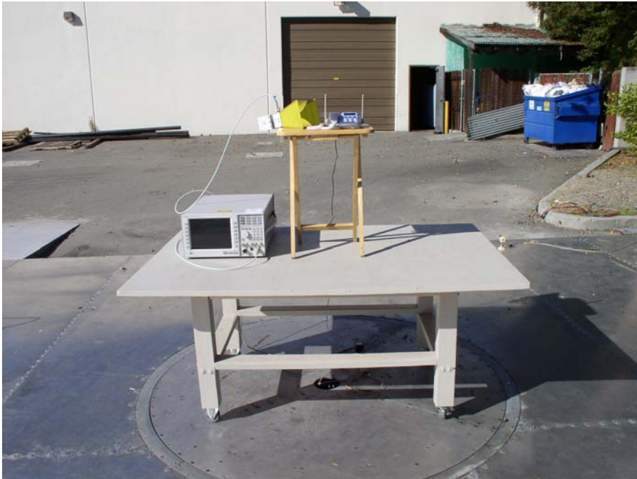
Base Radiated Emission – Front View (GSM)
