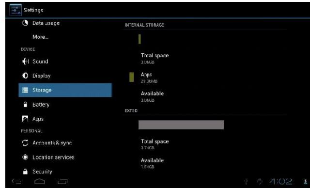
Check device memory and microSD card status. Unmount SD card – Unmount the SD card for safe removal.
