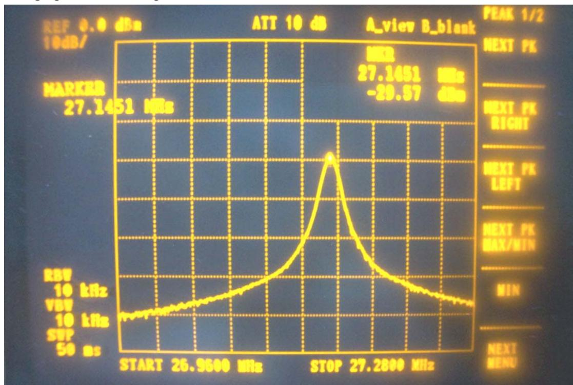
**The results: The unit does meet the FCC Part 15 C Section 15.227 requirements.**
