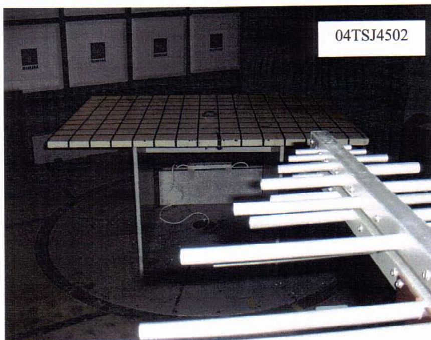
Photograph of test setup : Radiated Emission
