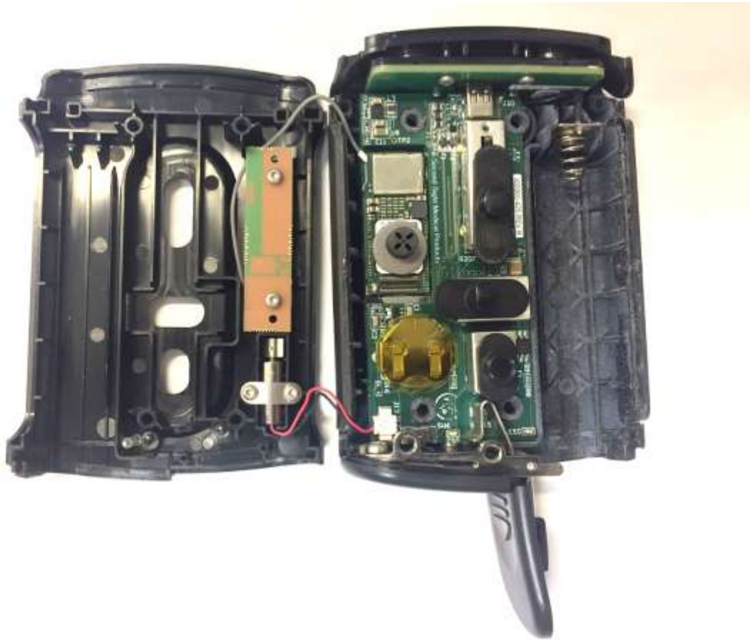
Fig 1.1. Interior view of VPU, showing component placement
