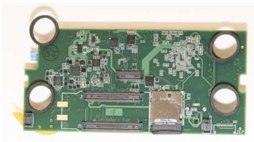
Fig 2.2. Part ENG 300300 663 VPU Main II Board Top (Auxiliary and SOM Boards Removed)
