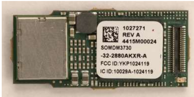
Fig 2.6. ENG 300300-608 SOM Board, Top (The Wi-Fi and Bluetooth functions are disabled)
