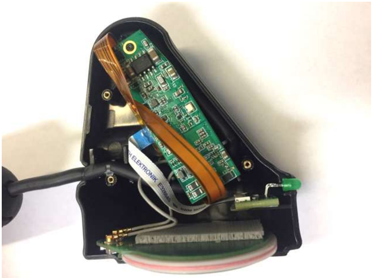
Fig 1.2. Interior view of the Operating Room (OR) wand showing RF electronics and antenna coil
