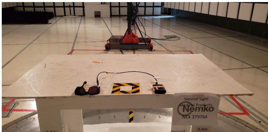
Figure 9.2.12 Radiated emissions 30-1000 MHz (Back)
