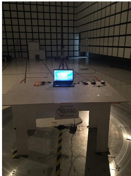
Figure 9.2.10 Radiated emissions 9 kHz-30 MHz (Test antenna at 90 deg, Back)
