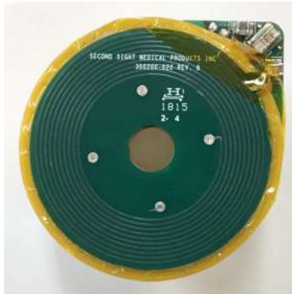
Fig 2.10. ENG-300200-029 RF Coil Sub-Assembly, Top)
