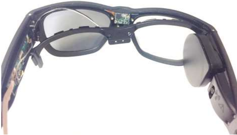
Fig 1.3. Glasses interior showing camera placement
