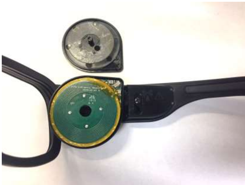
Fig 1.4. Glasses interior showing antenna coil placement
