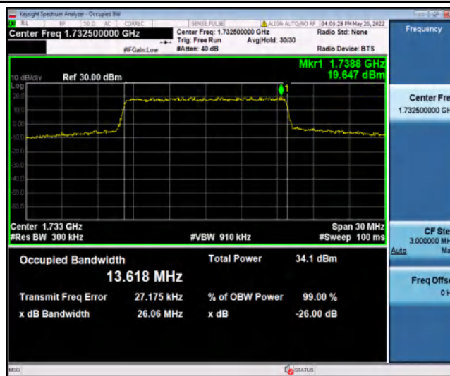
Band4-15MHz-QPSK-20175-75RB#0-13.618
