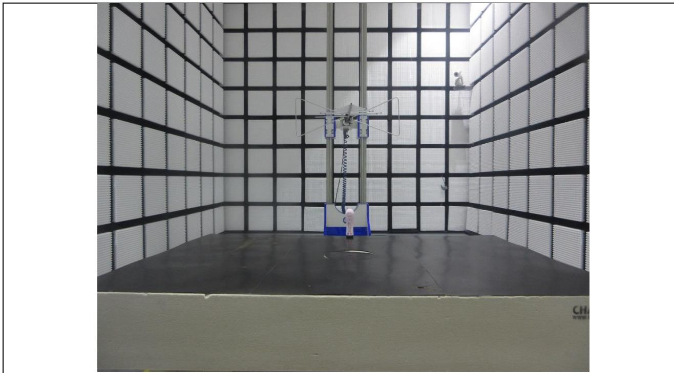
**Radiated Emission Test (1GHz – 18GHz)**
